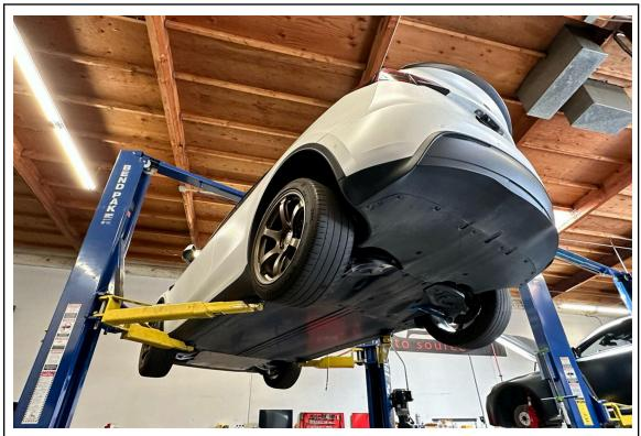
1. To install this skid plate, you will need to access the rear underside of the vehicle. Be sure to follow Tesla's lifting procedures to prevent damaging the battery and take extra precautions whenever working underneath the vehicle.
