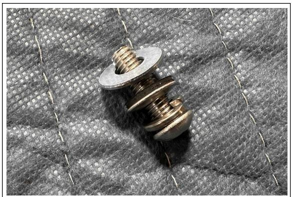
10. Using the image above for reference, slide a split lock washer onto a 20mm long bolt, then the metal/rubber washer with the rubber side facing out. Next, slide an M6 flat washer onto the bolt. Repeat for both 20mm long bolts.
