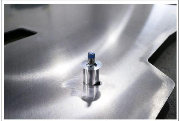
15. Apply 1-2 drops of the provided thread locker to each of the ten bolts.
