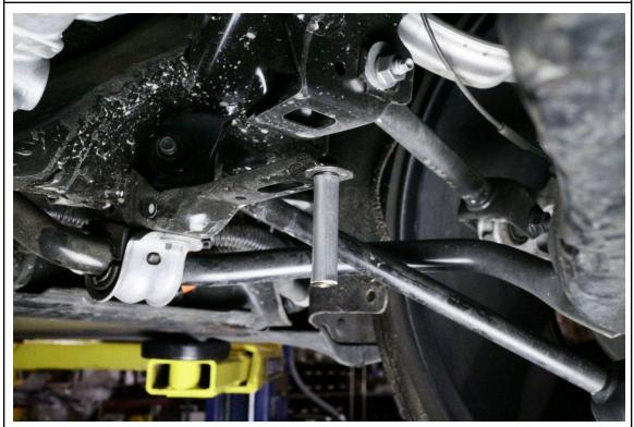
5. Apply 1-2 drops of the provided threadlocker onto the male end of the two provided threaded couplers. Install one onto each of the factory undertray mounting locations located just rear of the sway bar brackets. Once they are fully threaded on, use pliers to apply leverage to ensure the couplers are fully secured.
