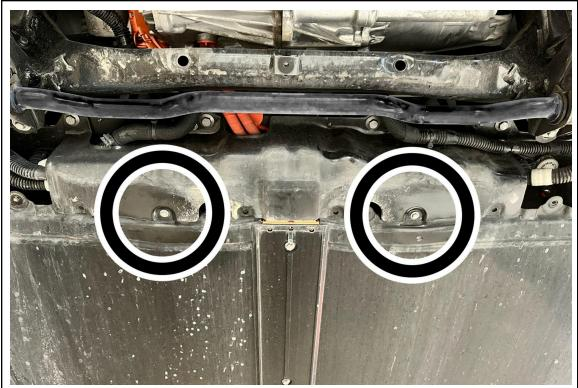
14. Clean the area surrounding the two bolts indicated in the image above. Cut the remaining piece of vinyl foam strip into two separate 2 inch pieces and apply it onto the bolts highlighted in the image.
