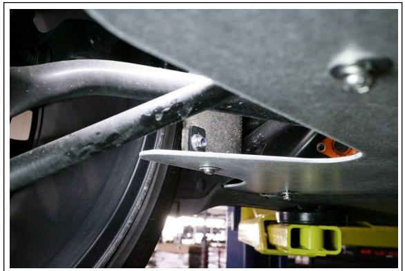
17B. If your vehicle had plastic clips securing the wheel well liner to the stock undertray, bolt the long end of the "L" bracket onto the wheel well liner using one of the provided 15mm M6 bolts, two flat washers, and nut. Then, bolt the short end of the "L" bracket to the skid plate using another short M6 bolt, two flat washers, and nut. Repeat for the opposite side.
