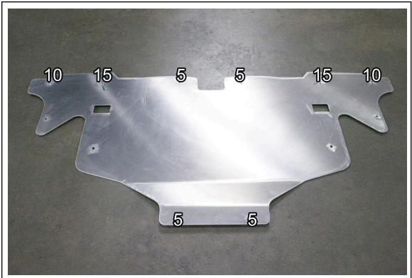
8. Slide the provided spacers onto the bolts. The numbers on the image indicate the thickness of the spacers in millimeters.
