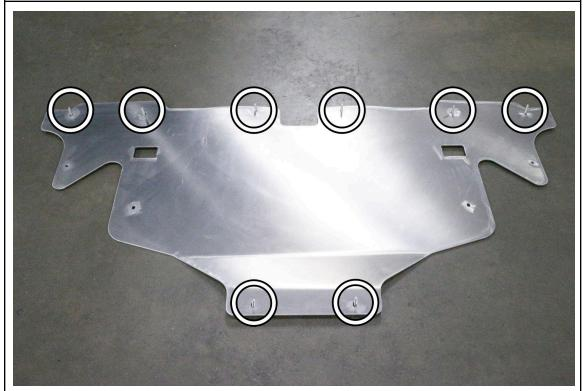
7. Place a piece of cardboard or a moving blanket large enough to fit the skid plate. Lay the skid plate flat with the logo side facing down. Insert the eight assembled bolts through the mounting points indicated above.
