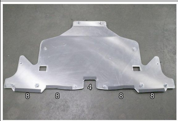
13. Cut the provided vinyl foam strip into the exact lengths shown on the image. The number indicates the length in inches. Use isopropyl alcohol to clean the areas on the skid plate where the vinyl foam strips will be installed. Apply the vinyl foam strips as shown. Stay within  $\frac{1}{6}$ " or 3mm from the edge of the skid plate.
