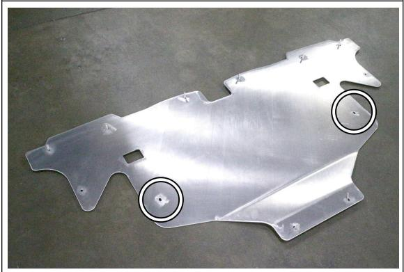
11. Insert the two assembled 20mm long bolts into the two holes indicated above, in the same orientation as the previously installed bolts.
