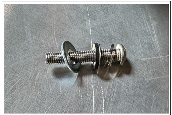
6. Using the image above for reference, slide a split lock washer onto a 35mm long bolt, then the metal/rubber washer with the rubber side facing out. Next, slide an M6 flat washer onto the bolt. Assemble a total of 8 sets.
