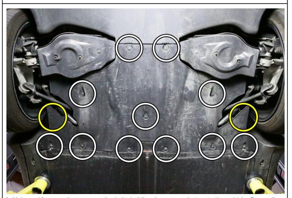
3. Using a 10mm socket, remove the bolts holding the rear undertray to the vehicle. Depending on the year and model, there are a total of either 11 or 13 bolts.
