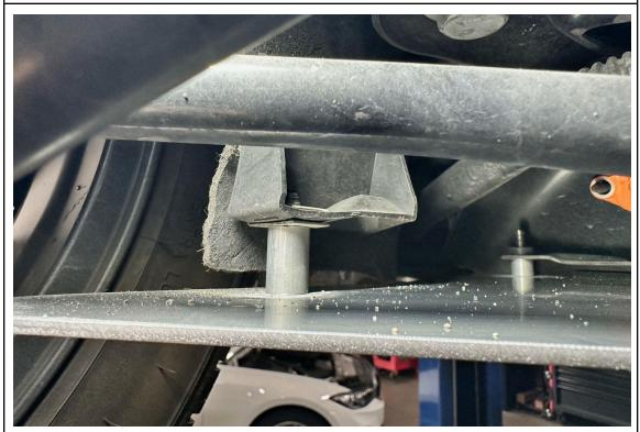
17A. If your vehicle had bolts securing the wheel well liner to the stock undertray, place a 20mm long spacer onto the top side of one of the remaining holes on the skid plate. Insert one of the provided 35mm long M6 bolts and a flat washer through the skid plate to secure the wheel well liner to the skid plate. Repeat for the opposite side.
