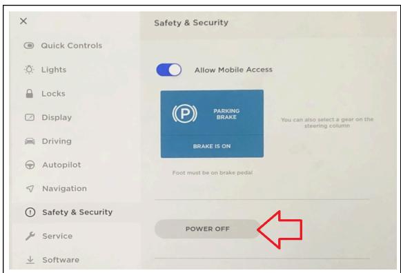
2. Power off the vehicle through the touch screen by tapping "Menu" > "Safety and Security" > "POWER OFF".
