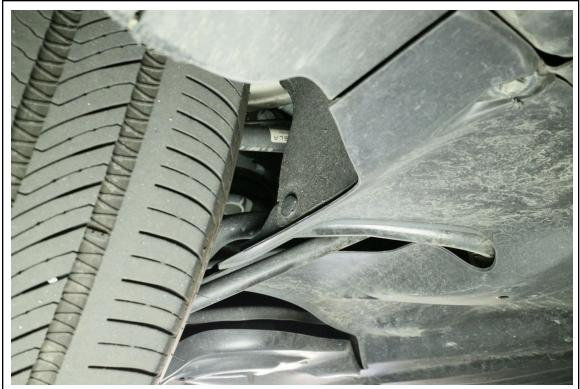
4. If your vehicle only had 11 bolts securing the undertray, you will need to locate one clip on each side of the vehicle securing the wheel well liner to the undertray. Once the clips have been removed, the undertray can be removed from the vehicle.
