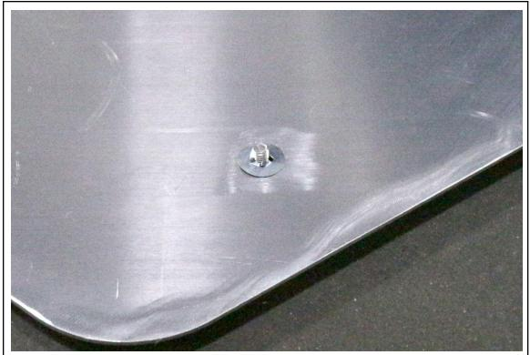
12. Install a round push nut onto each of the two 20mm bolts to capture it onto the skid plate.
