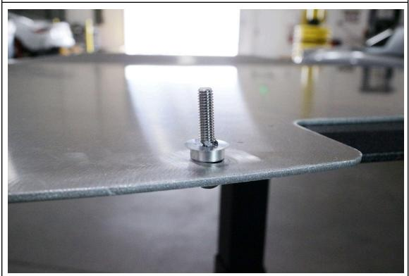
9. Once the spacers are in place, install a round push nut onto each bolt to capture the hardware to the skid plate.
