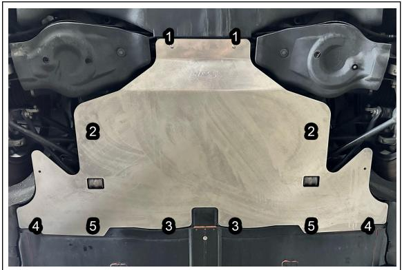
16. Thread on the bolts in the sequence shown, working in pairs. Leave the bolts loose to allow for adjustability until all of the bolts are threaded.
