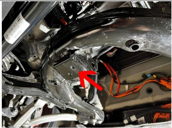
4. Install the provided bracket onto the mounting point located in the center of the subframe.
