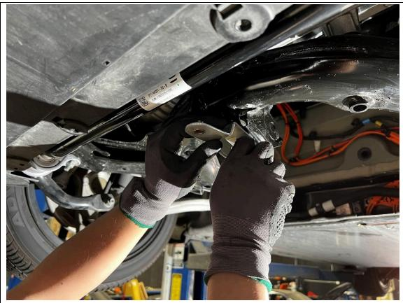
5. Position the bracket as shown with the threaded side facing the front of the vehicle. Secure the bracket to the subframe using one of the included M6 screws and stainless steel washer.
