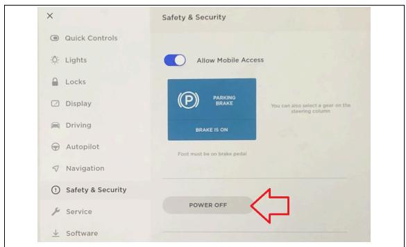
1. Power off the vehicle through the touch screen by tapping "Menu" > "Safety and Security" > "POWER OFF".
