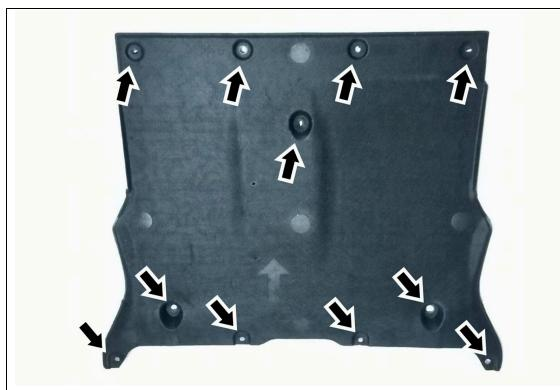
3. Lift the vehicle to access the front undertray. Use a 10mm and 15mm socket to remove the stock undertray.
