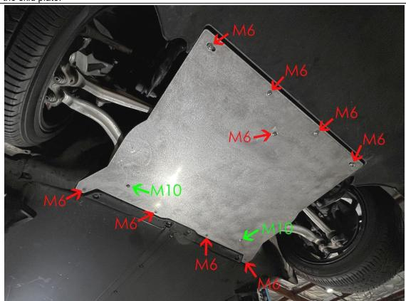
8. Install the provided bolts in their designated locations as shown above. For the M6 screws, install a stainless steel washer between the screw and skid plate.
