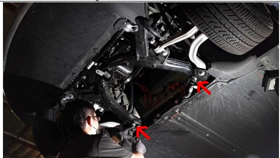
6. Install the M10 coupling nuts onto the large studs at the rear of the subframe. Use a 17mm socket and torque wrench to tighten to 35 ft-lb.
