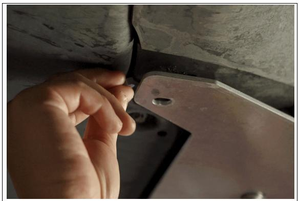
7. Add the two provided spacers on the rear corner mounting points between the vehicle and the skid plate.
