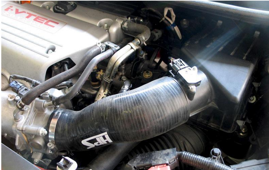
This is how the HPS Silicone Tube Installed:
