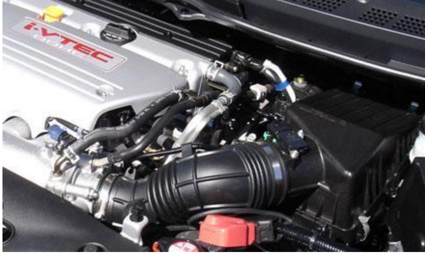
This is how the stock intake hose looks like:
