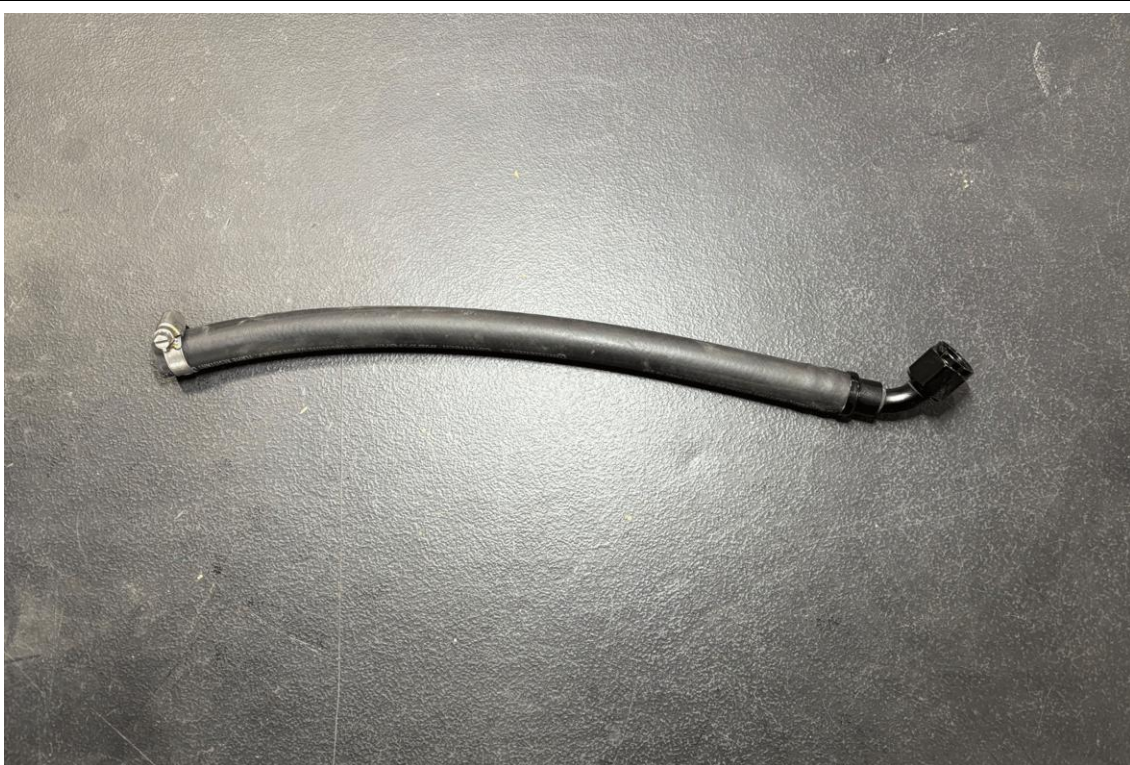
13. Assemble the provided -8 hose, -8 fitting, and embossed hose clamp as shown above.
