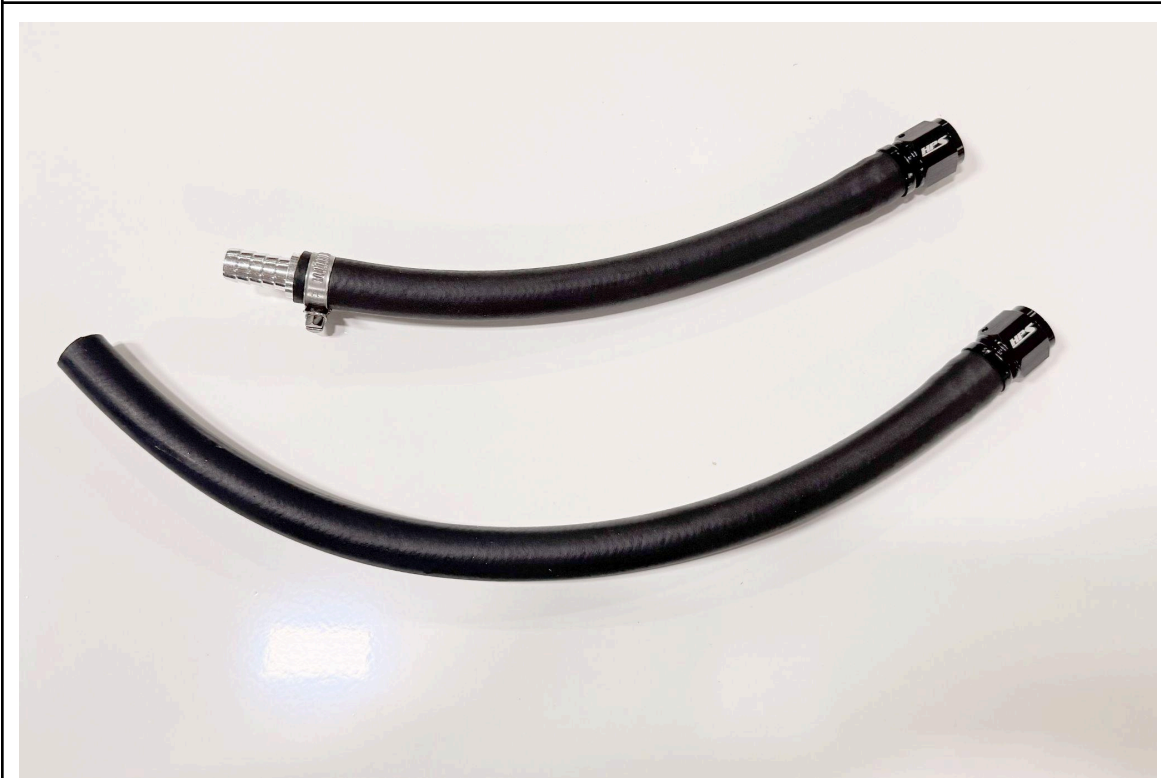
12. Install the AN hose end fittings onto the hoses as shown. On the shorter hose, install the provided 1/2" barbed fitting and secure it using one of the provided embossed hose clamps.
