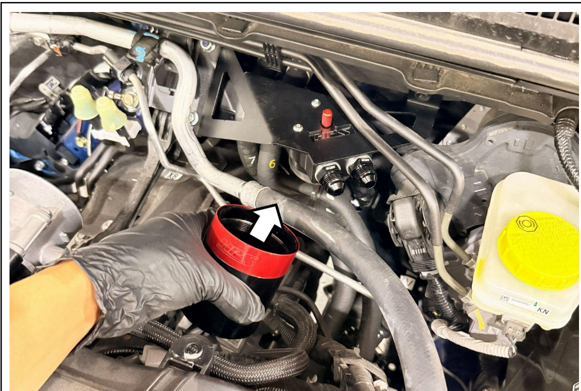
11. Reinstall the can back onto the catch can housing.
