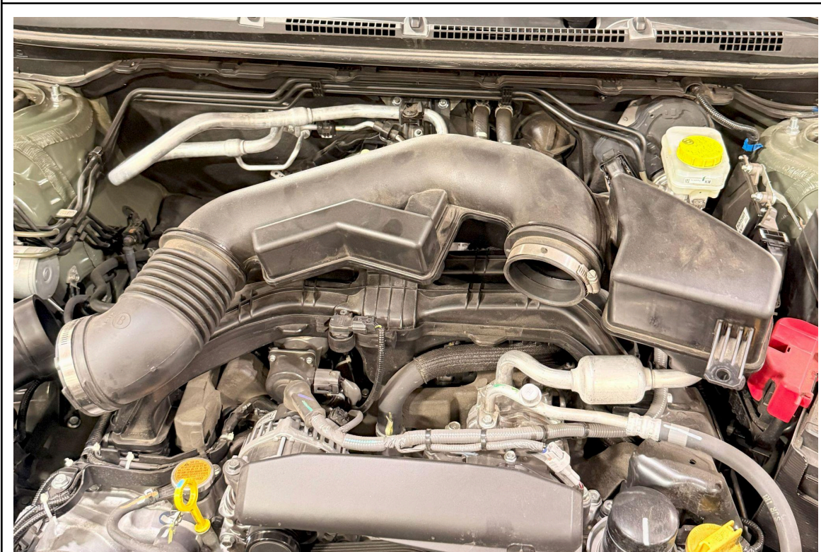
4. Disconnect the air intake tube from the air cleaner box and throttle body.
