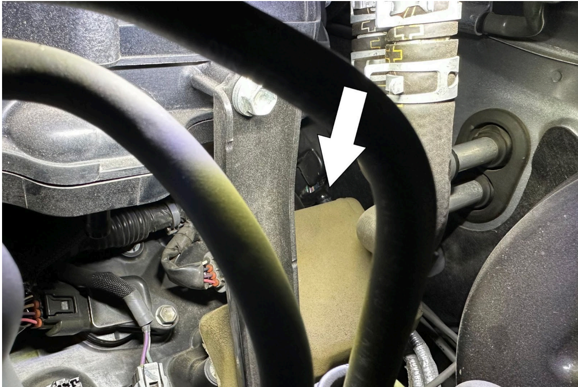
9. Install the opposite end of the shorter AN hose onto the PCV barb.
