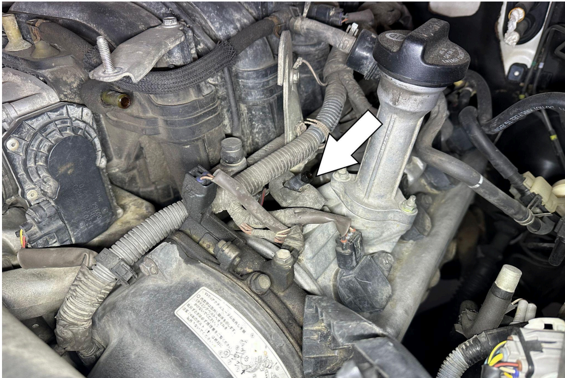
11. Install the opposite end of the shorter hose to the PCV barb.
