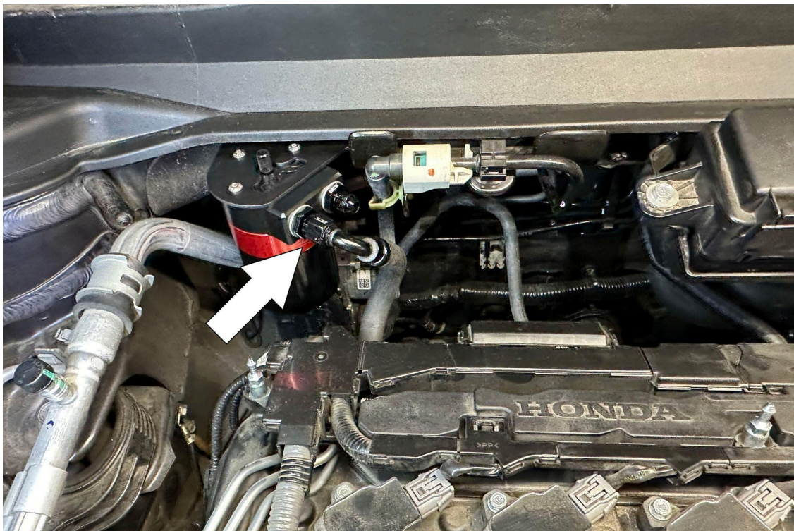
12. Install the 7.5-inch long hose to the fitting that is closest to the engine.
