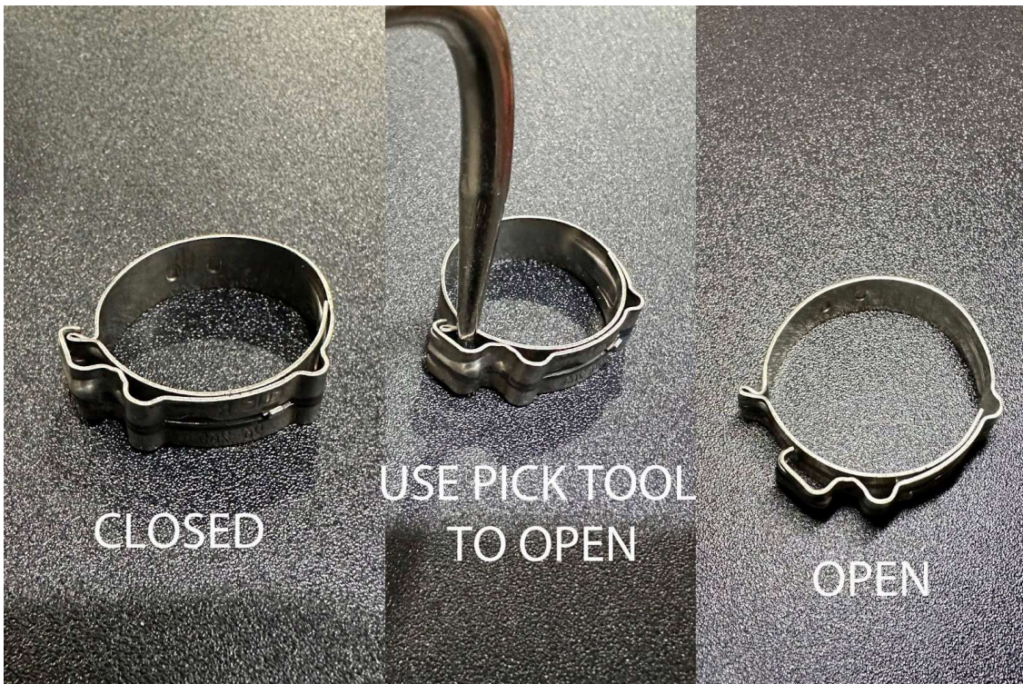
12. The picture above shows how to open the original PCV valve clamp. The original clamp will be reused when installing the new hose.
