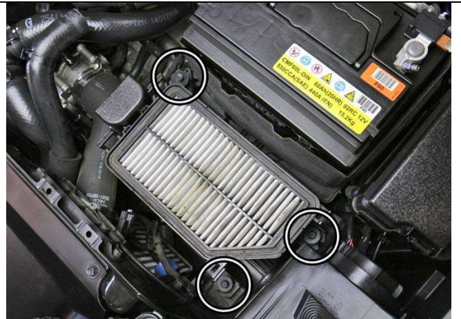
9. Loosen and remove the three bolts from the lower part of the air box using a 10mm socket.
