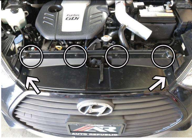
16. Remove the four 10mm bolts and the two plastic clips indicated in the image above.
