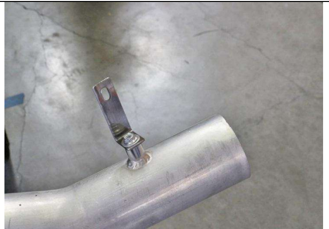
28. Install the "L" shaped intake bracket onto the cold air intake pipe.
