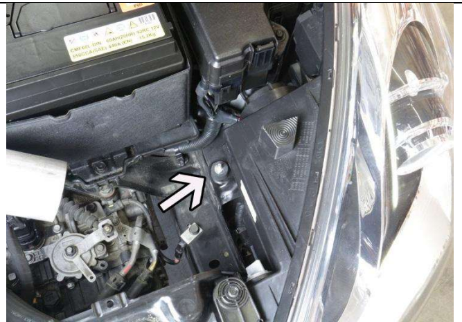
25. Install the 1/2 rubber vibration mount onto the stock air box mount located in the image above.
