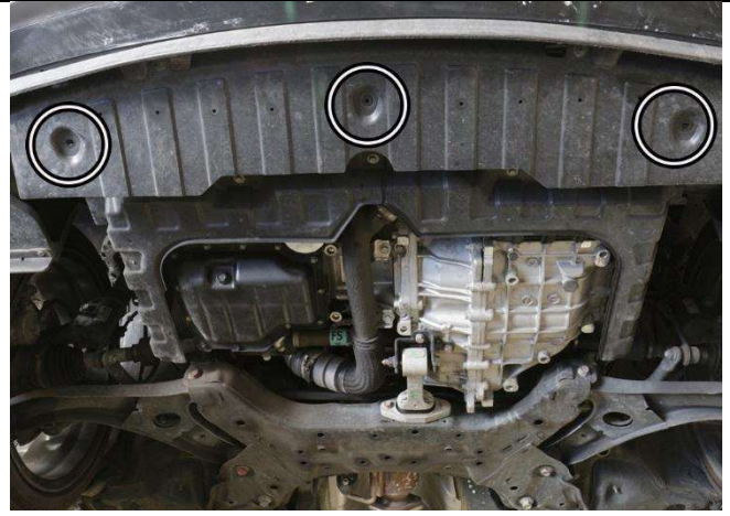
17. Remove the three 10mm bolts securing the lower part of the bumper.
