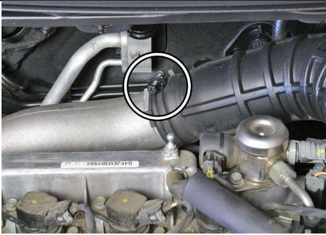
4. Loosen the hose clamp securing the intake tube to the turbo inlet.
