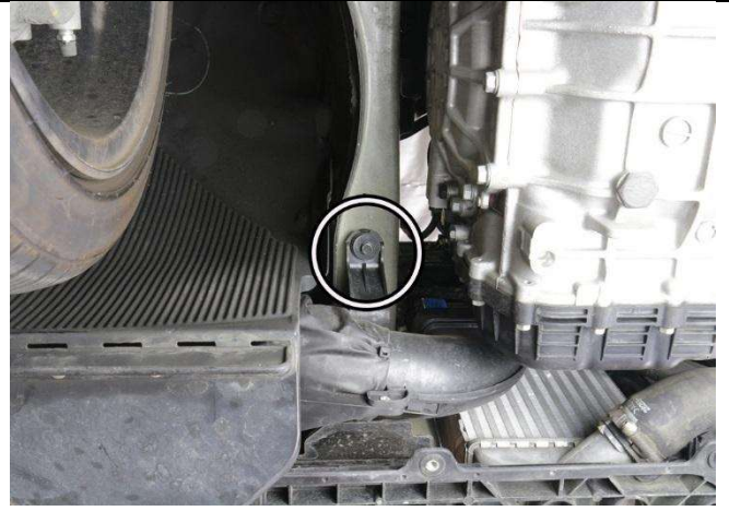
23. Remove the last 10mm bolt securing the lower resonator assembly.
