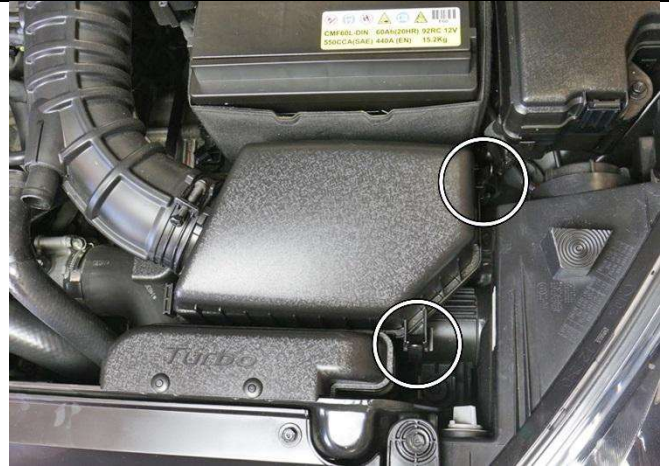
5. Unclip the two retaining buckles from the air box.
