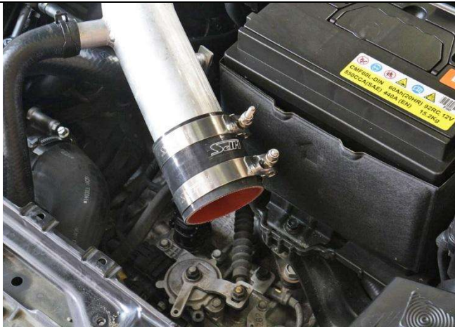
27. Insert the straight silicone coupler along with T-bolt clamps onto the HPS intake pipe.
