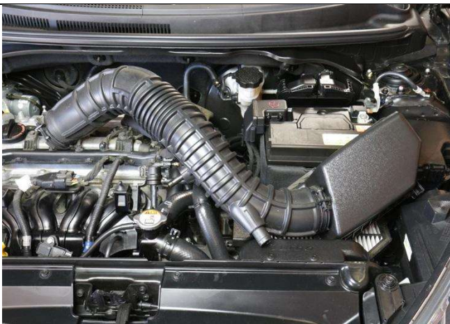
6. Remove the stock intake tube assembly as well as the top portion of the air box from the vehicle.
