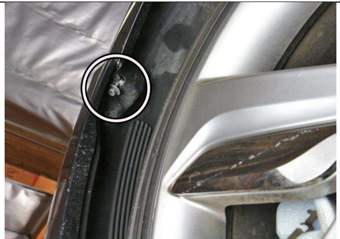
19. Remove the 10mm bolts located at the driver side and the passenger side inner wheel liner. Remove the front bumper slowly and disconnect the fog light connectors freeing the bumper from the vehicle.
