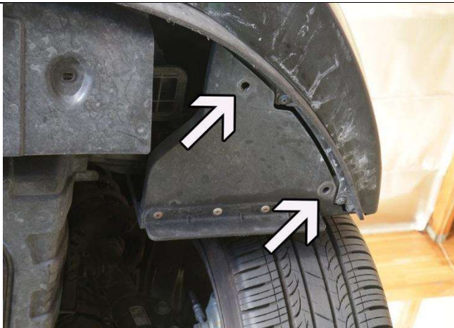
18. Remove the two plastic clips from the lower driver side fender well loosening the liner from the bumper.
