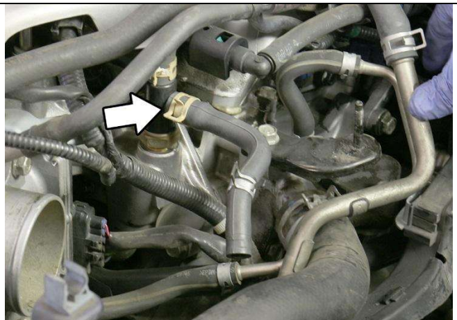
13. Disconnect and remove the hose indicated using needle nosed pliers to release the clamp.
