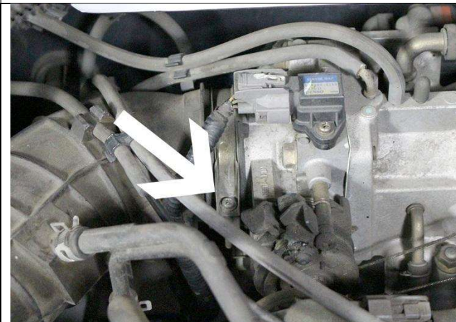
4. Use a phillips head screwdriver to loosen the hose clamp on the throttle body.
