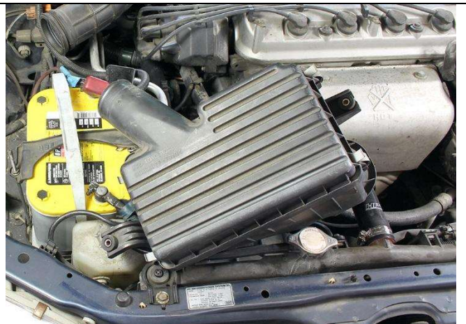
3. Separate the air box from the stock rubber intake tube and remove it from the engine bay.
