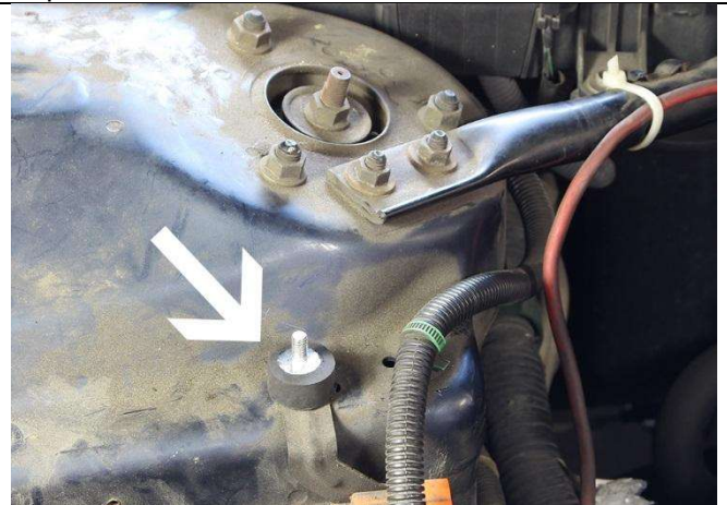
10. Remove the factory bolt in the location indicated using a 10mm socket, then replace the bolt with a M6 x 1/2" rubber vibration mount from the hardware pack.
