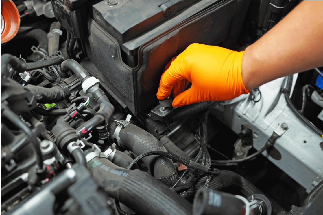
11. Install one of the provided 1/2" vibration mounts onto the factory air box mounting hole.
