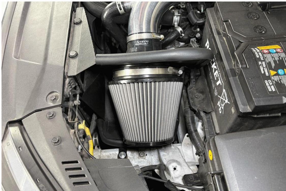
20. Secure the provided HPS Performance Air Filter onto the velocity stack.
