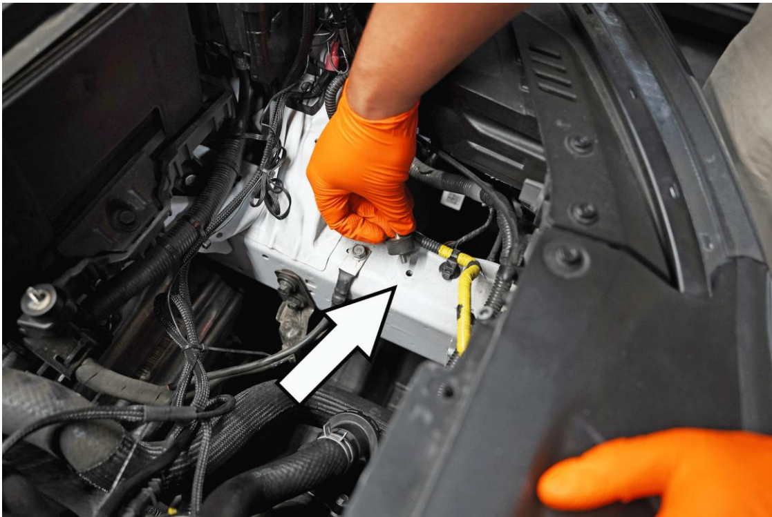
12. Install the second 1/2" vibration mount onto the other factory air box mounting hole.
