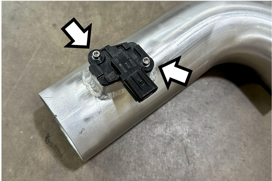
13. Secure the MAF sensor onto the HPS intake pipe using the two provided M4 bolts.
