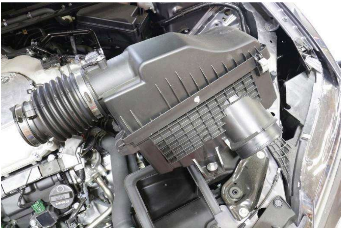
8. Remove the intake hose from the throttle body and remove the air box assembly from the vehicle.
