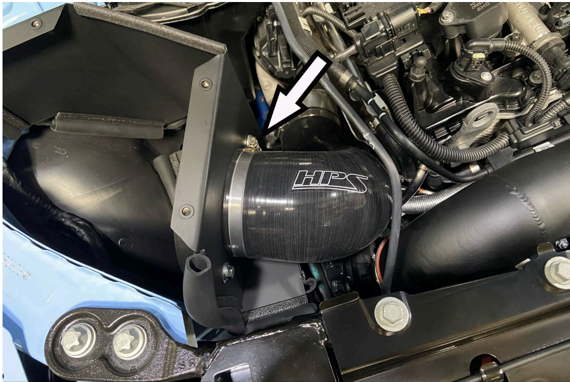
25. Secure the HPS silicone intake hose onto the velocity stack.
