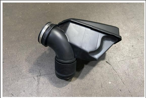
9. Remove the factory intake hose and resonator from the vehicle.
