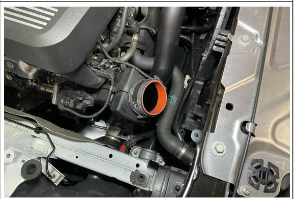
10. Install the silicone coupler onto the turbo inlet pipe using the two provided EMSC clamps. Tighten the clamp on the turbo inlet pipe and leave the second clamp loose to fit the intake pipe in later steps.
