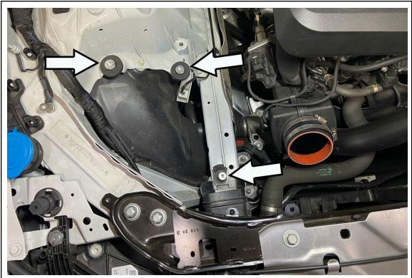
11. Install the three provided M6 mounting bungs into the factory rubber grommet mounts.
