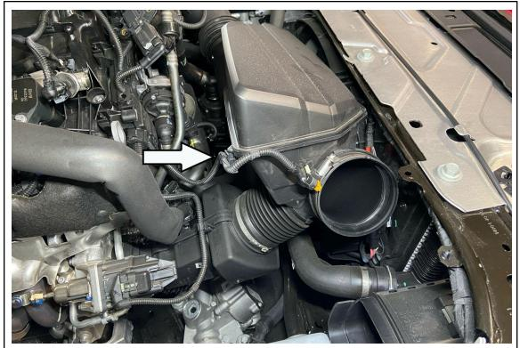
7. Unclip the MAF electrical harness from the resonator on the intake hose.
