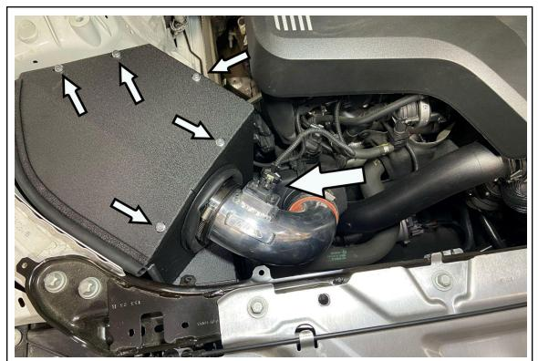
17. Secure the lid onto the heat shield using the five provided M5x12mm bolts. Reconnect the MAF sensor electrical connector.
