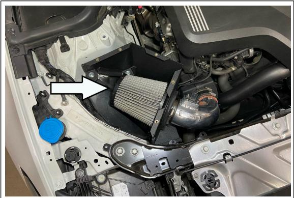
15. Insert the HPS intake pipe into the silicone coupler and install the provided air filter as shown.
