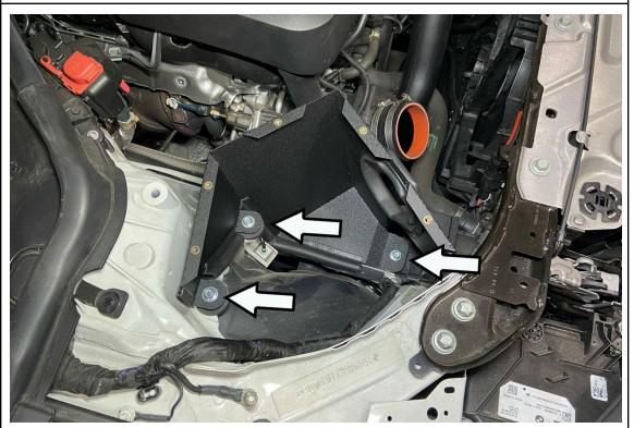
14. Secure the HPS heat shield onto the M6 mounting bungs using the three provided M6x12mm bolts and washers.
