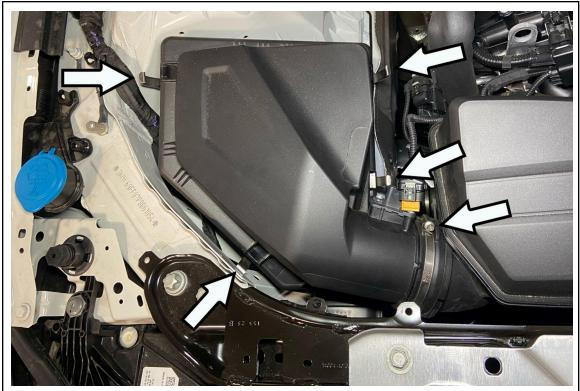
3. Disconnect the four retaining clips on the air box assembly. Loosen the hose clamp securing the intake hose to the air box.
