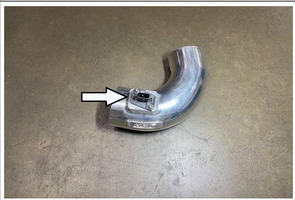
12. Remove the mass air flow sensor from the factory upper air box and secure it to the HPS intake pipe using the two provided M4 Allen bolts.
