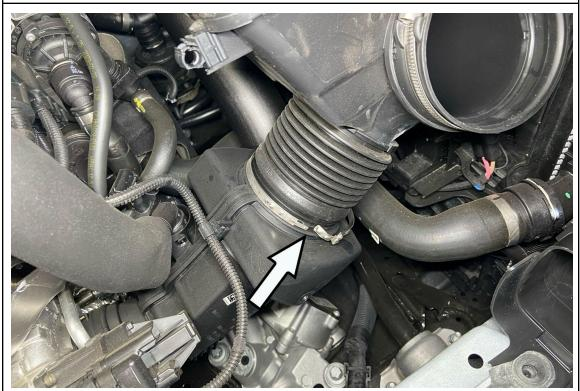
8. Using a flat head, pry off the locking tab to unclip the hose clamp securing the intake hose to the turbo inlet pipe.
