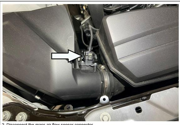
2. Disconnect the mass air flow sensor connector.
