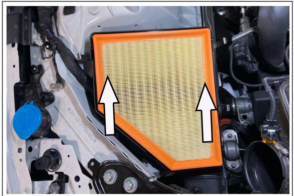
5. Lift firmly on the lower air box to release it from the mounting grommets.
