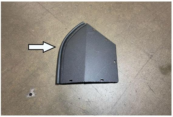
16. Cut and install the bubble edge trim onto the heat shield lid.
