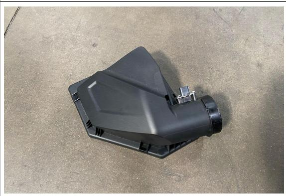
4. Remove the upper air box from the vehicle.
