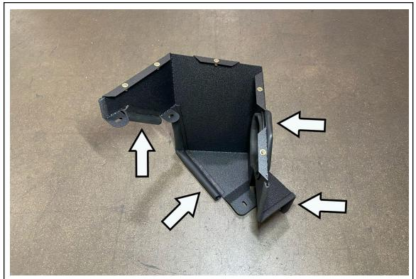
13. Cut and install the provided bubble edge trim and thin edge trim onto the HPS heat shield as indicated above.
