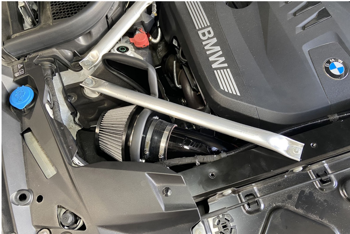
21. Reinstall the factory tower brace.
