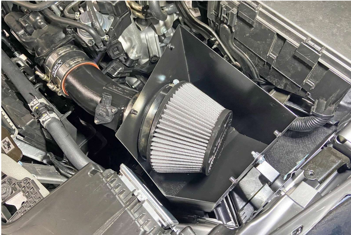
17. Install the HPS performance air filter onto the velocity stack.
