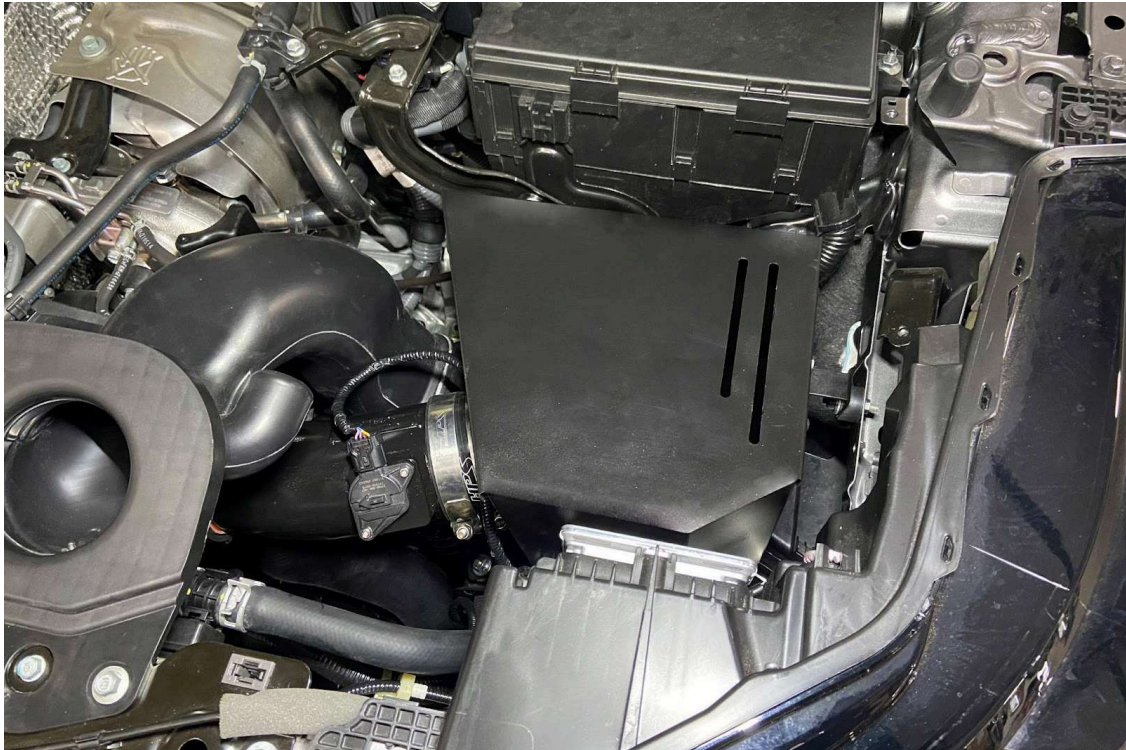
21. Secure the heat shield lid with the provided M5 x 12mm bolts (4).
