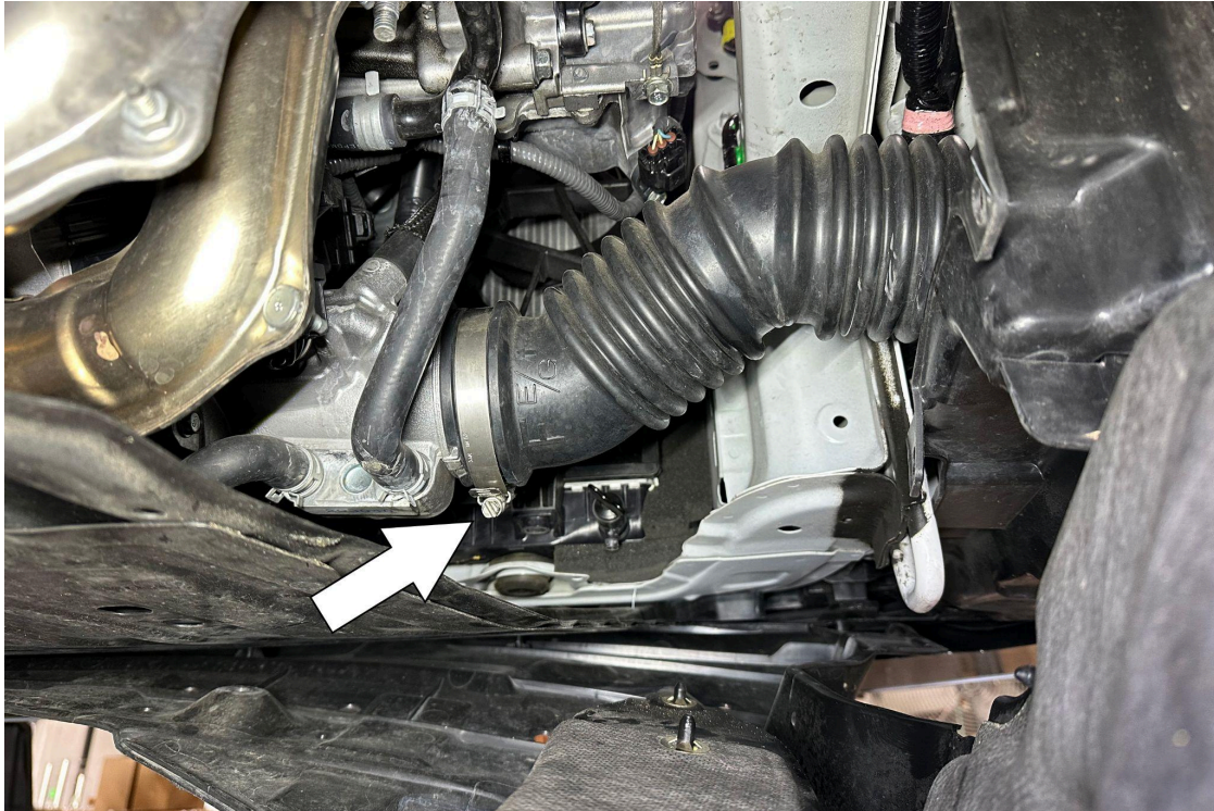
9. Loosen the hose clamp securing the intake tube to the turbocharger inlet, then remove the intake tube from the vehicle.
