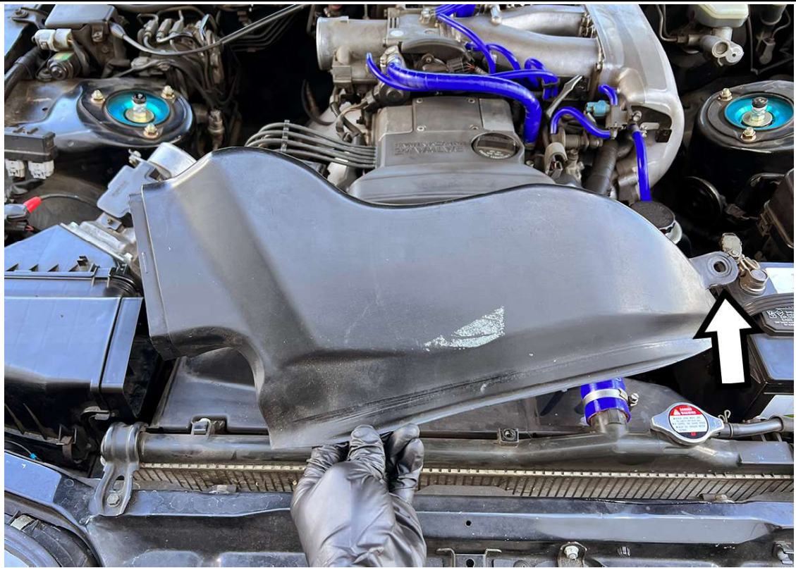
9. Loosen the 10mm bolt and remove the air inlet duct at the front of the vehicle.
