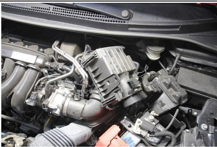
6. Disconnect and remove the upper air box assembly from the factory intake tube.
