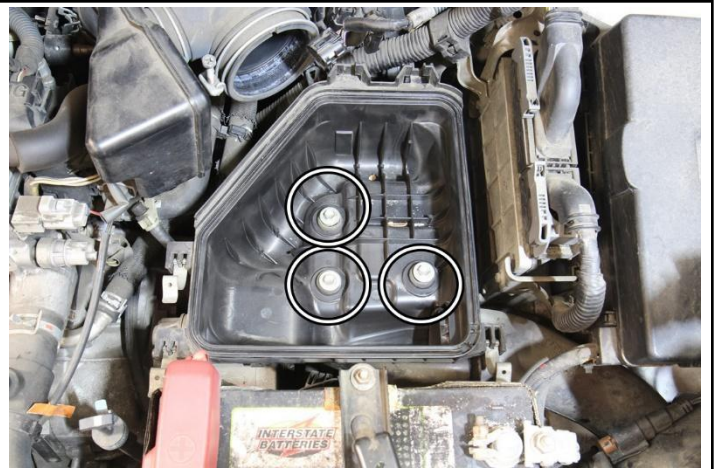
9. Remove the three 10mm bolts securing the lower air box.
