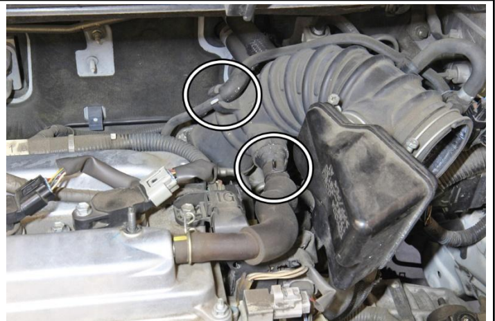
11. Disconnect the breather crank case hose from the intake tube and remove the EVAP hose from the intake tube.
