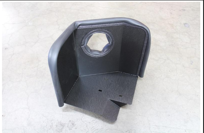
23. Insert the bubble edge trim onto the heat shield.
