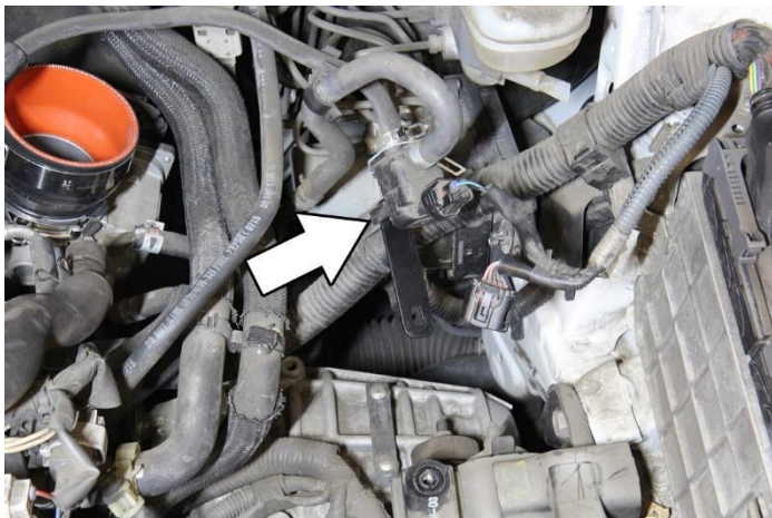
16. Install and secure the provided bracket onto the EVAP solenoid by using the factory screw and the M5 washer included in the hardware kit.
