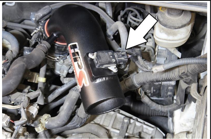
21. Reinsert the MAF sensor harness back into the MAF sensor.
