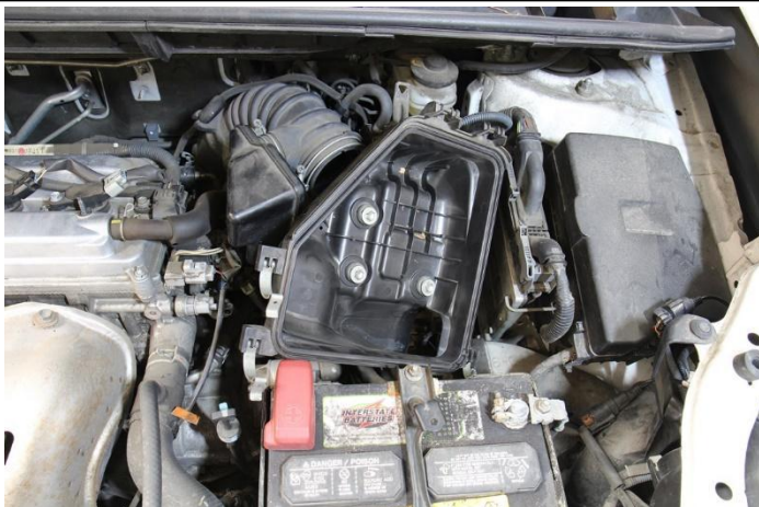
10. Disconnect the lower air box from the air duct tube and remove the lower air box from the vehicle.
