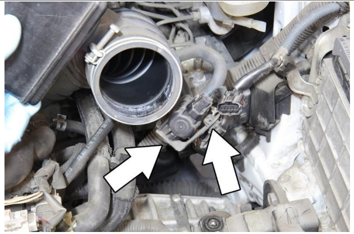
13. Remove the screw securing the EVAP sensor from the bracket, then depress the harness clip to remove to completely remove the electrical harness from the intake tube.
