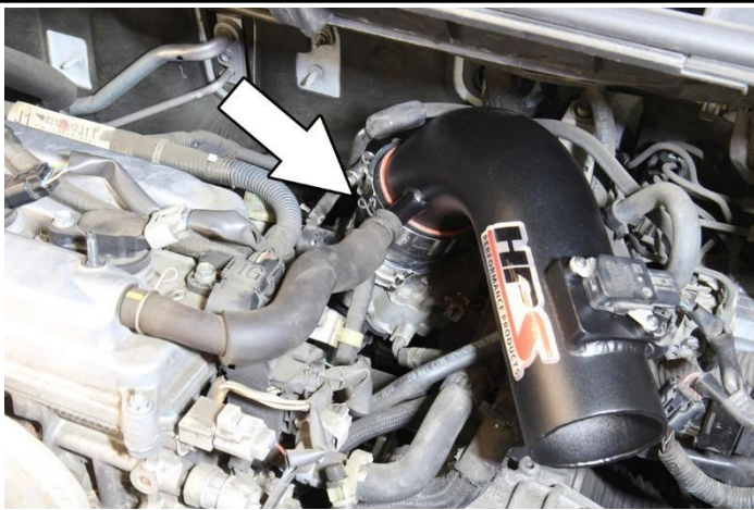
20. Reinstall the factory breather hose to the intake barb.
