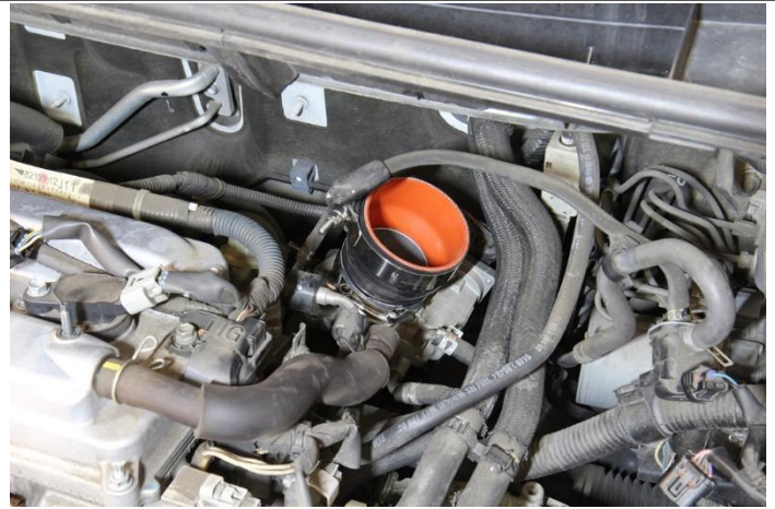
15. Install the reducer coupler along with the provided T-bolt clamps onto the throttle body.
