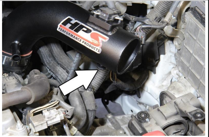
19. Secure the EVAP solenoid bracket to the intake pipe using the provided M6 x 12mm bolt and washer.
