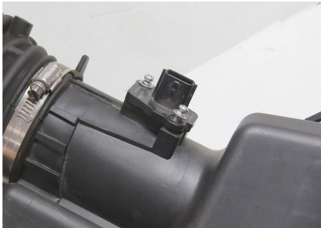
14. Use a Phillips screwdriver to remove the MAF sensor from the stock upper air box.
