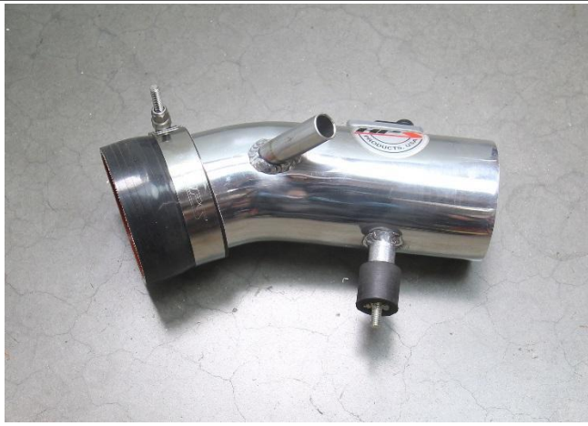
16. Thread the rubber vibration mount onto the threaded bung on the HPS intake pipe.
