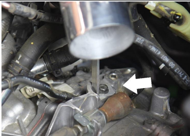
20. Install the intake bracket onto the rear shifter bracket hole reusing the original bolt.
