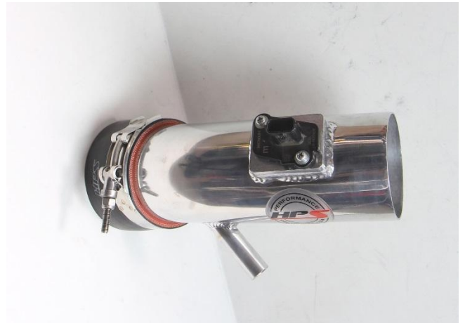
15. Transfer the MAF sensor onto the HPS intake pipe and secure it using the stock screws.
