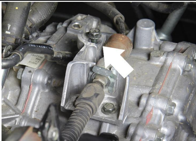
18. Loosen and remove the rear shifter bracket bolt on the transmission. Do not discard the bolt as it will be used again later.
