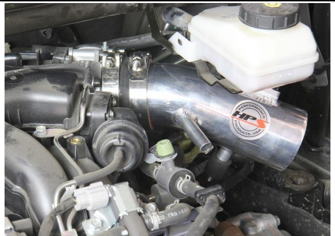
19. Insert the HPS intake pipe onto the throttle body. Lightly secure the T-bolt clamp onto the throttle body.
