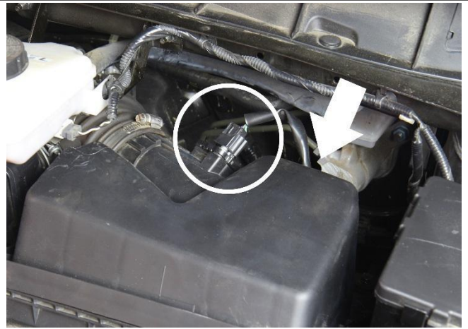
5. Disconnect the MAF sensor connector. Locate and unclip the cable tie at the back of the air box.
