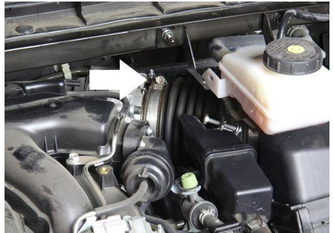
7. Loosen the hose clamp on the throttle body using a flat head screw driver. Once loose, the stock intake hose can be disconnected.
