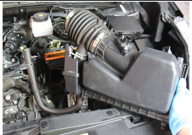
9. Remove the upper air box from the engine bay.
