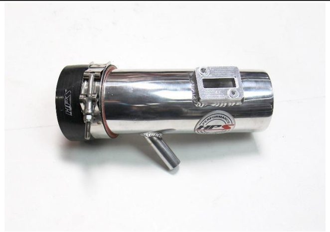
13. Connect the silicone reducing coupler onto the intake pipe as shown. Be sure to not let the pipe go past the step on the inside of the coupler. Secure the T-bolt clamp when the coupler is in the desired position.
