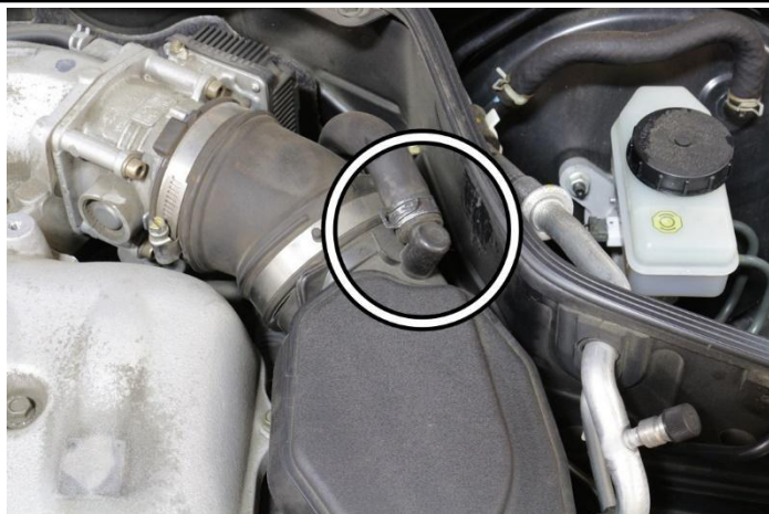
4. Loosen the hose clamp securing the breather hose from the intake tube.
