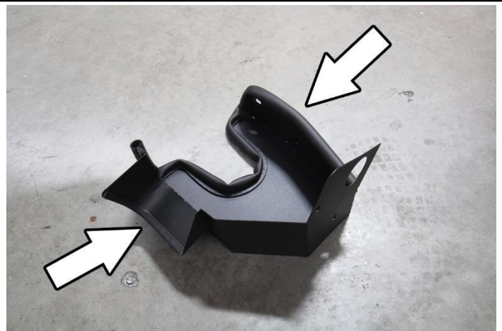
11. Insert the thin edge trim provided in the hardware kit indicated from the left arrow shown above onto the heat shield. Insert the bubble edge trim onto the heat shield indicated from the arrow on the right shown above.
