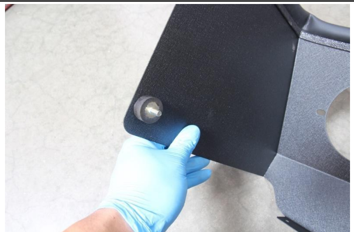
15. Install and secure the provided vibration mount into the slot of the heatshield using a M6 nut and washer.
