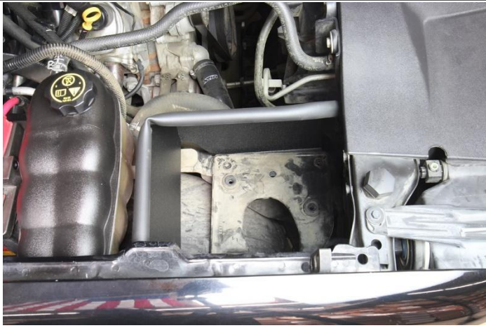
16. Slide the heatshield underneath the factory air box mount and re-use the bolts that were removed in steps 13 to secure the heatshield.
