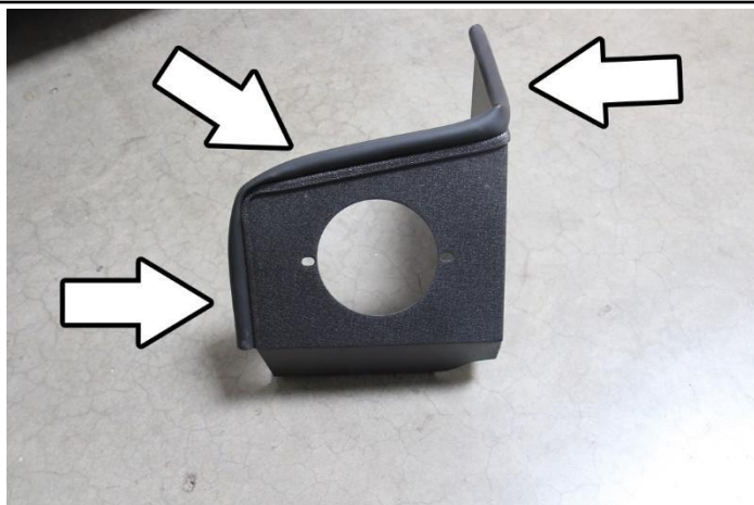
14. Install the bubble edge trim onto the heatshield.
