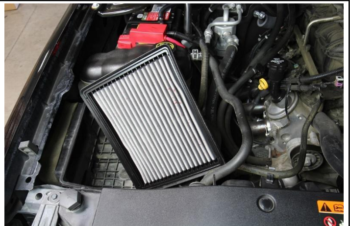
9. Remove the air filter from the vehicle.
