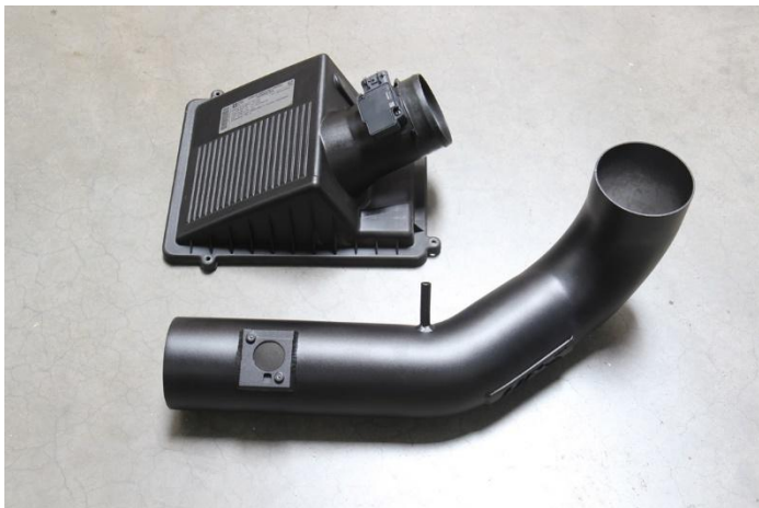
18. Install the mass air flow sensor onto the HPS intake pipe using the provided M4 bolts.
