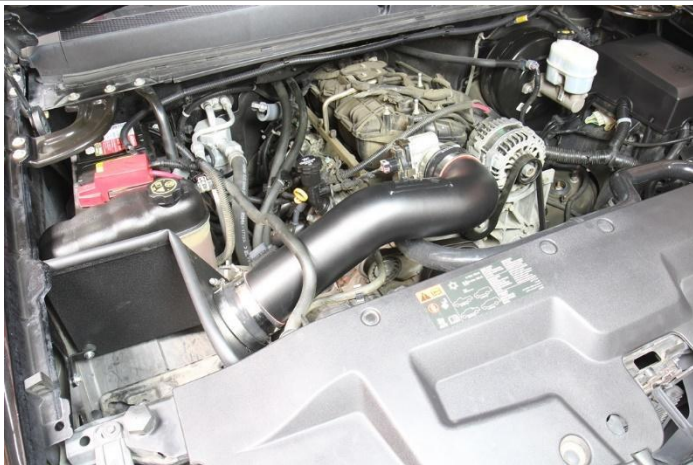
20. Insert the HPS intake pipe into the throttle body coupler.
