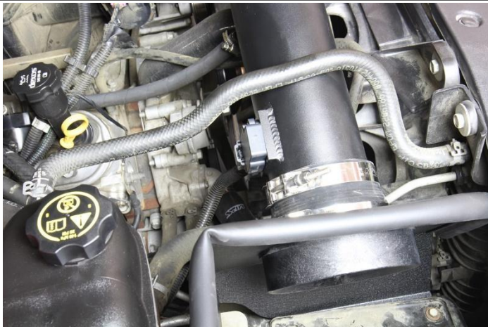
24. Re-connect the MAF sensor harness connector.
