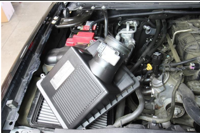
8. Remove the upper air box assembly from the vehicle.
