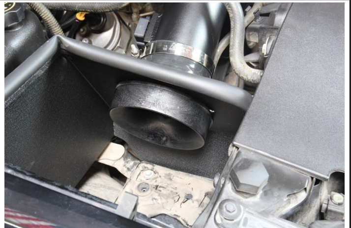
21. Insert the velocity stack onto the intake pipe and secure the velocity stack to the heatshield using the two M6 x12mm bolts and washers.
