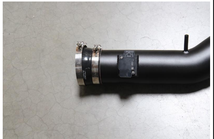
19. Slide on the provided reducer coupler onto the end of the pipe near the MAF sensor, but do not secure any of the clamps yet.
