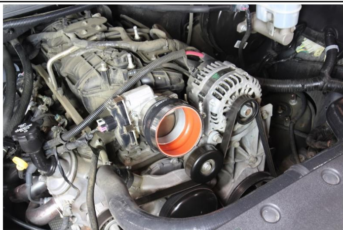
12. Insert the hump coupler onto the throttle body along with the provided T-bolt clamps.
