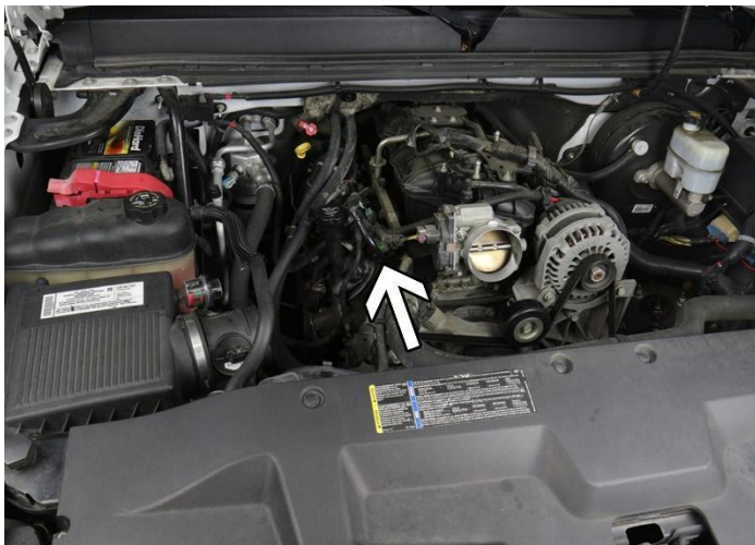
6. Rotate the breather line to unclip and remove the air line from the valve cover.
