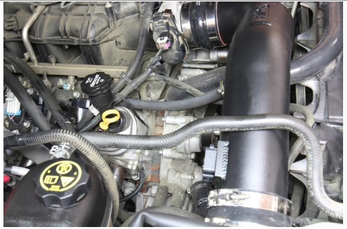
23. Insert the provided EPDM hose onto the breather barb of the pipe and the valve cover. Secure the hose using the two EMSC clamps.
