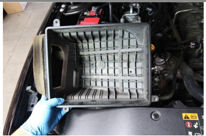
11. Remove the lower air box assembly from the vehicle.
