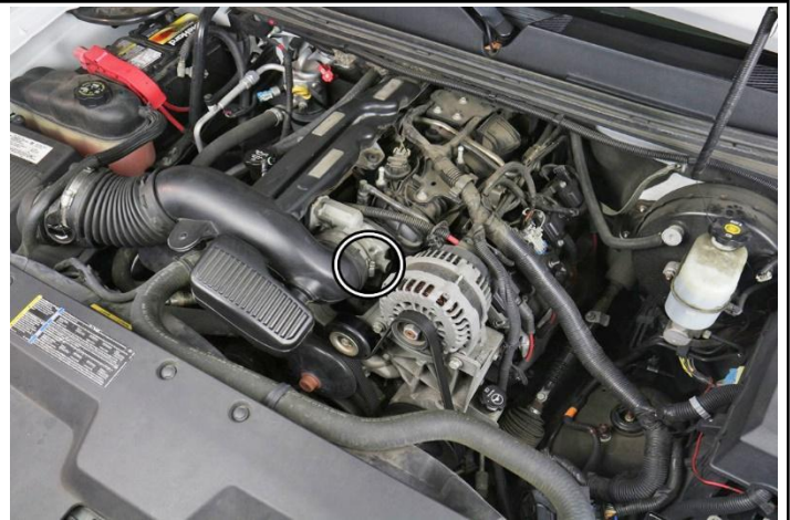
5. Loosen the hose clamp securing the intake tube from the throttle body and remove the stock intake tube from the vehicle.
