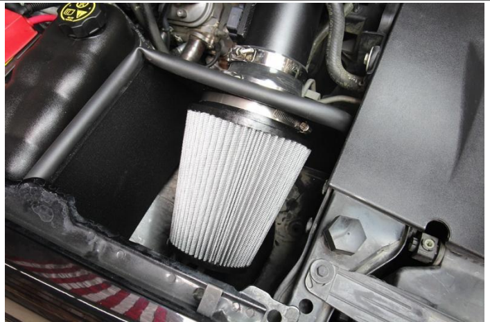
25. Install the HPS Performance air filter.
