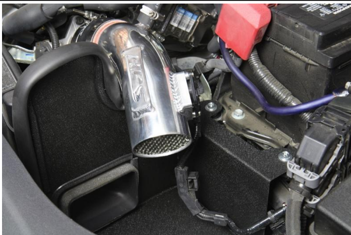
20. Reconnect the MAF sensor harness connector onto the MAF sensor.
