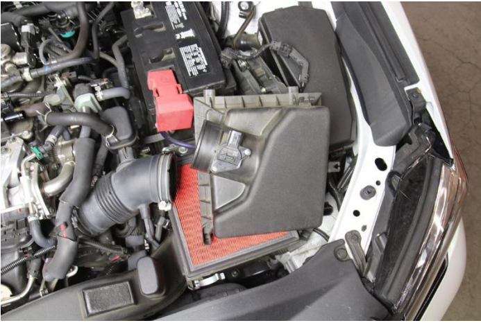
7. Remove the upper air box assembly from the intake tube.
