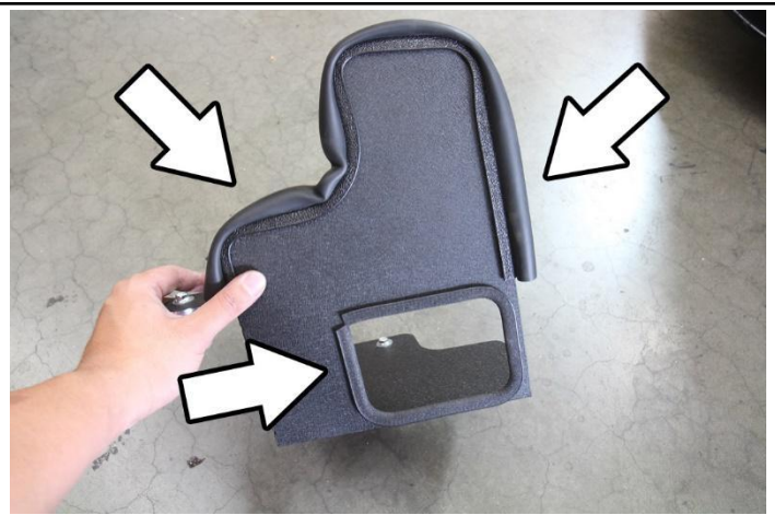
13. Install the bubble edge trim onto the top portion of the heat-shield and the thin edge trim onto the air scoop opening.
