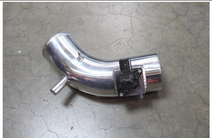
15. Remove the stock MAF sensor from the upper air box assembly and install it on the HPS intake pipe. Secure the sensor using the two M4 Allen bolts provided in the hardware kit.
