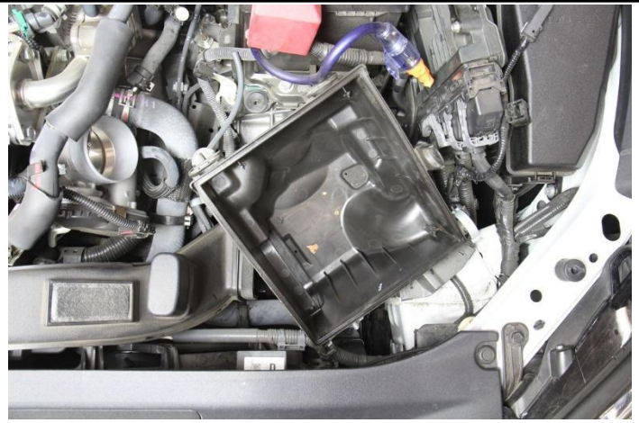
11. Lift and remove the three mounts from the lower air box assembly from the rubber grommets.
