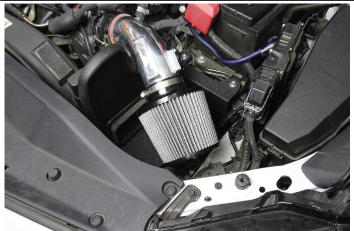
21. Install the HPS air filter onto the intake pipe.
