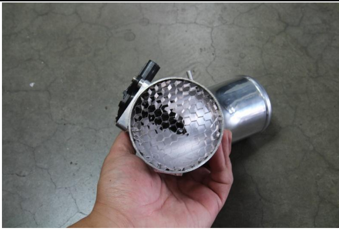
16. Insert the provided honeycomb into the intake pipe closest to the MAF sensor.
