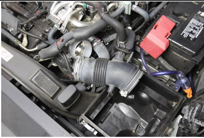
10. Remove the stock intake tube from the vehicle.
