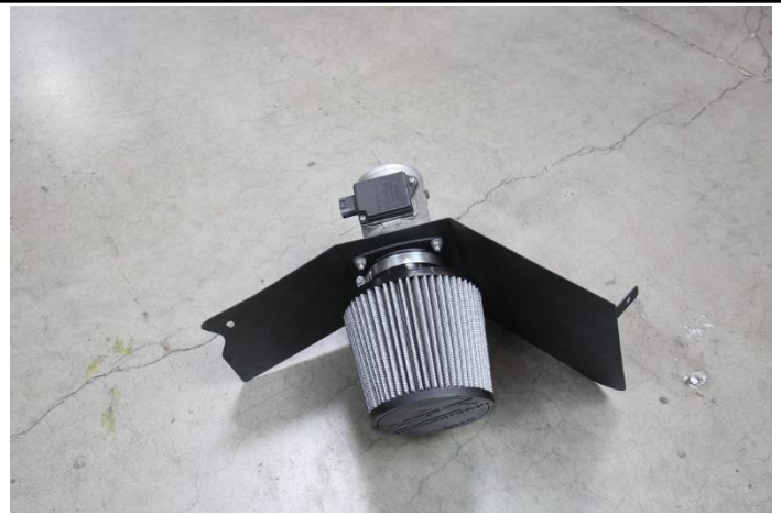
13. Mount the HPS air filter onto the MAF adapter on the front side of the heat shield.
