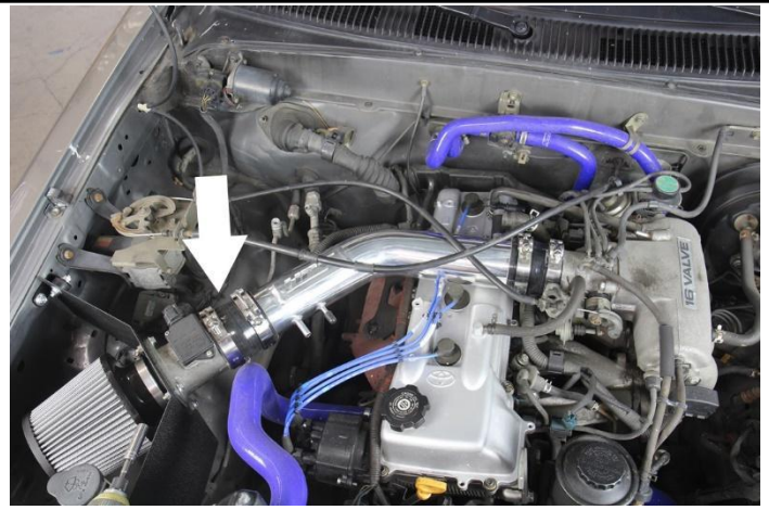
19. Tighten all intake hose clamps and anything else that may not be tight yet.
