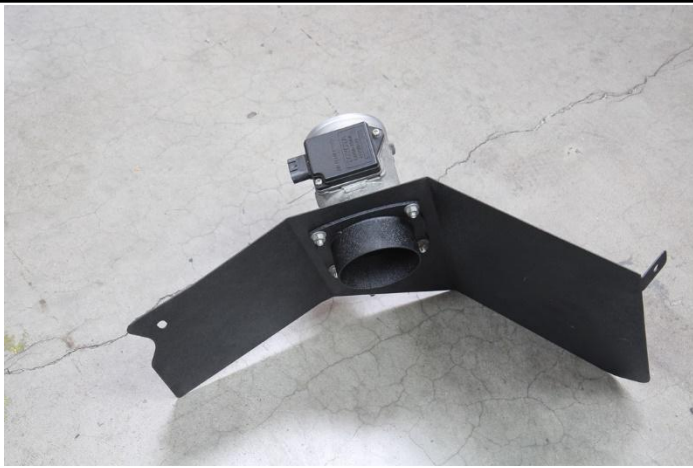
12. Mount the MAF with the rubber gasket on the back side of the heat shield with the MAF adapter on the front side of the heat shield.
