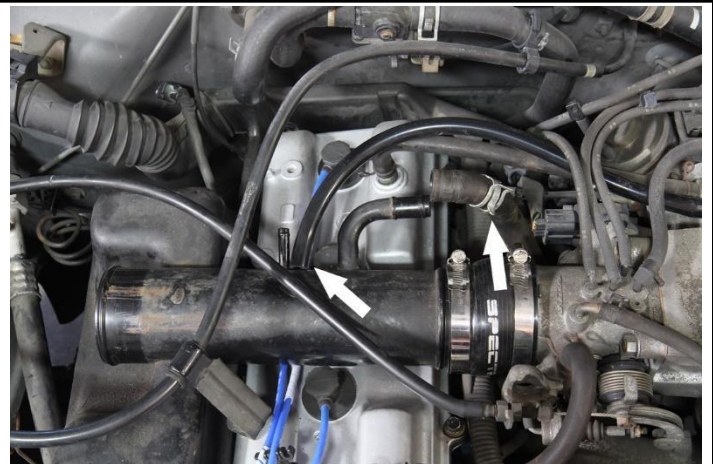
5. Remove the factory IACV hose(right) and the throttle body bypass hose(left) from the intake pipe.
