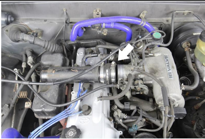
6 Loosen and remove the intake pipe from the throttle body. (pictured on the left side of this photo is the air resonator box, there are two nuts underneath it securing it to the engine.
