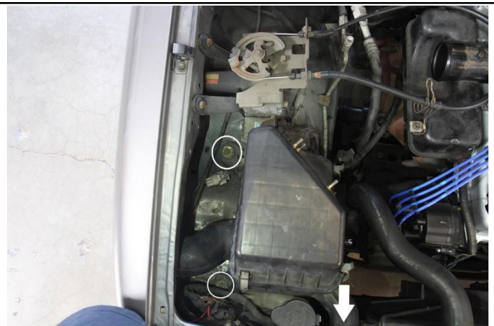
9. Remove the factory air box from the engine bay by removing the bolts shown above.
