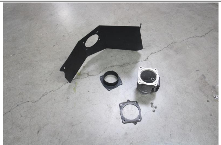
11. Gather the heat shield, MAF adapter, rubber gasket, factory m6 nuts and HPS supplied m6 30mm long bolts.
