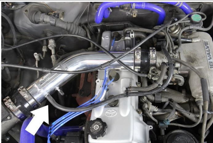
22. Install the other end of the vacuum hose onto the intake pipe.
