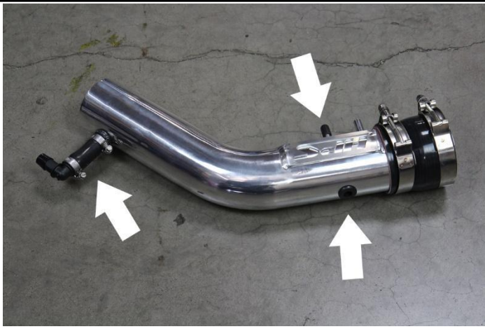
18. Install the 3/8" rubber grommet in the open intake hole. Install the 16mm vacuum hose onto the barb pictured with the 90 degree male to male barb facing parallel with the intake pipe and secure them together with the HPS provided clamps.
