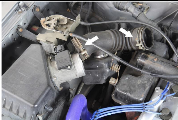
2. Loosen OEM hose clamps on each end of the intake hose.
