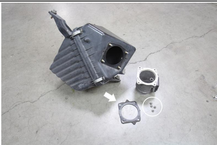
10. Using a 10mm wrench or socket, remove the MAF sensor and rubber gasket. Make sure to keep the factory m6 nuts as we're going to reuse them along with the rubber gasket.
