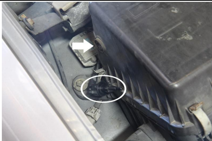
4. Remove the intake air temp sensor from the stock air box. Twist and pull with light pressure.
