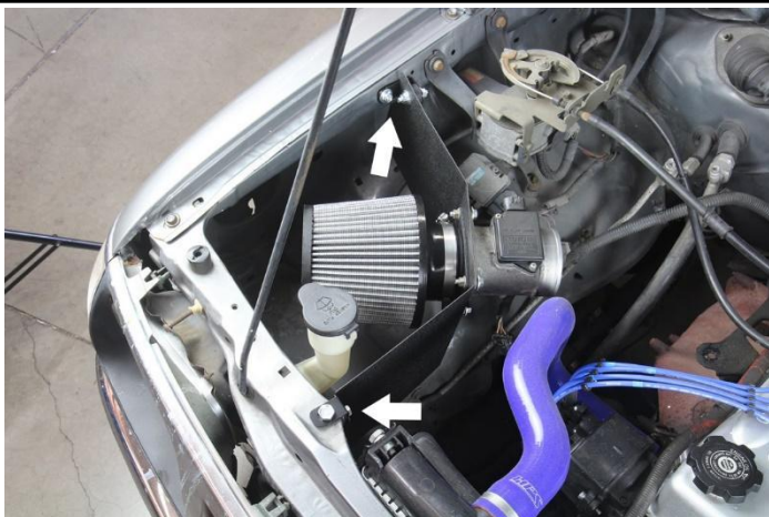
14. Slide the heat shield into the original air box section of the engine bay.
