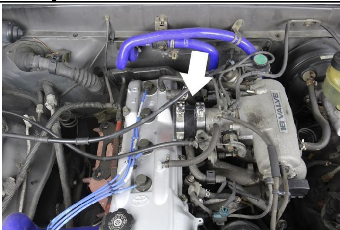
8. Install 2.75" to 3" HPS coupler with the supplied T-Bolt clamps to the throttle body.
