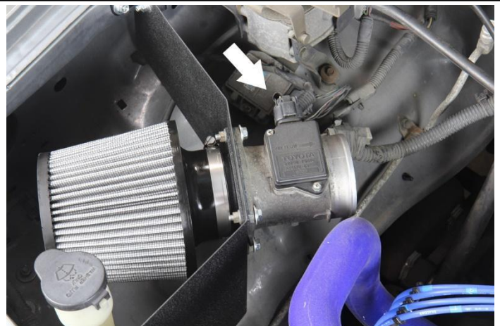
17. Reconnect the MAF sensor.
