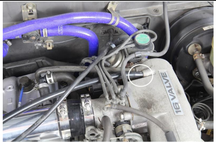
21. Install HPS supplied new vacuum hose onto the intake manifold barb circled.
