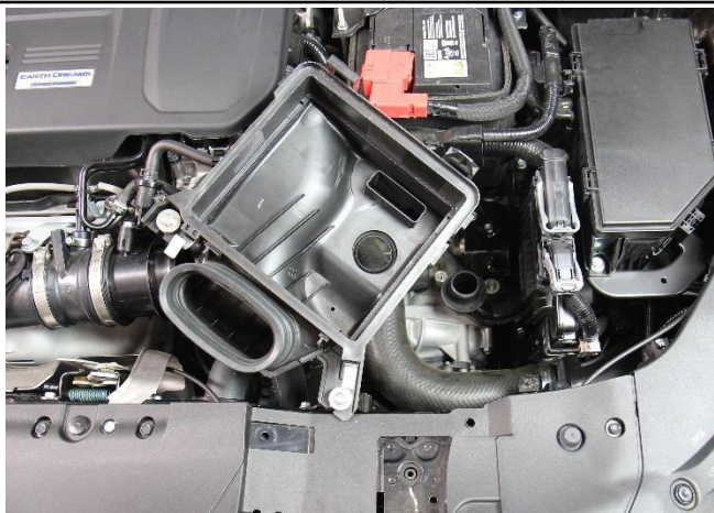
8. Remove the lower airbox from the engine bay.
