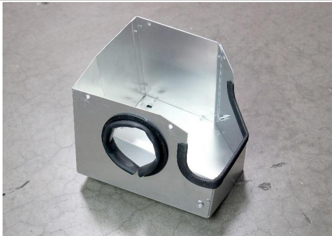
16. Install the provided edge trim as shown. Be sure to use the bubble edge trim in the circular opening and the narrow edge trim along the edge shown.
