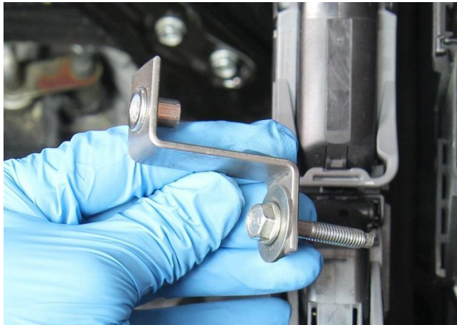
14. Use the bolt removed to attach it to the Z bracket provided.
