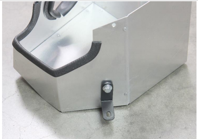
17. Loosely install the L bracket on the right side of the heat shield using a M6 x 16mm bolt and washer.
