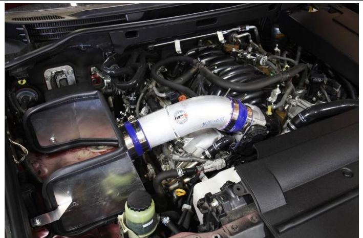
19. Install the stock MAF sensor onto the HPS intake pipe using the M4 screws provided. Then slide the other reducer coupler onto the other end of the intake pipe, but do not tighten the clamps yet. Insert the HPS intake pipe into the throttle body coupler.
