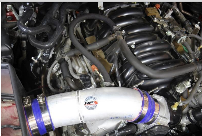
20. Connect the breather hose and the vacuum hose onto the intake barbs. Re-connect the MAF sensor harness connector onto the MAF sensor.
