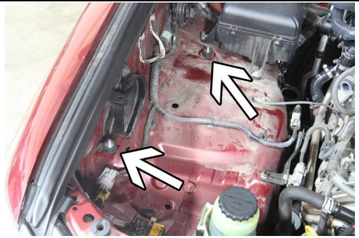
11. Install the two ½ inch vibration mounts shown in the indicated areas above.
