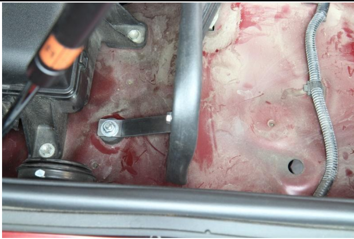
16. Align the bracket to the heat-shield and secure the bracket using the other m6 x 16mm bolt, nut, and washer.
