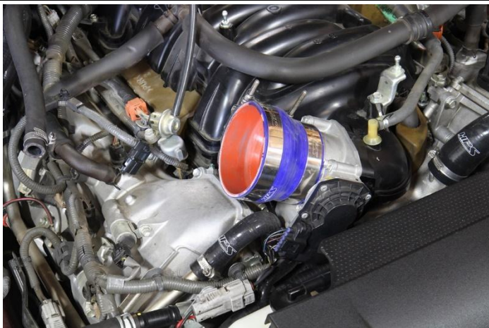
18. Install the provided 3.50" – 4.00" reducer coupler along with the t-bolt clamps onto the throttle body.
