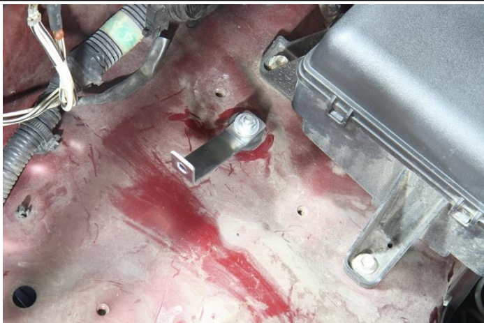
14. Install the other bracket onto the rubber vibration mount located near the back of the firewall.
