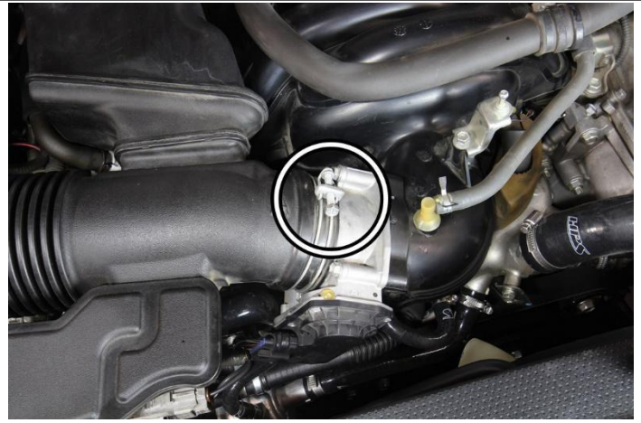
5. Loosen the hose clamp from the intake tube securing the throttle body.
