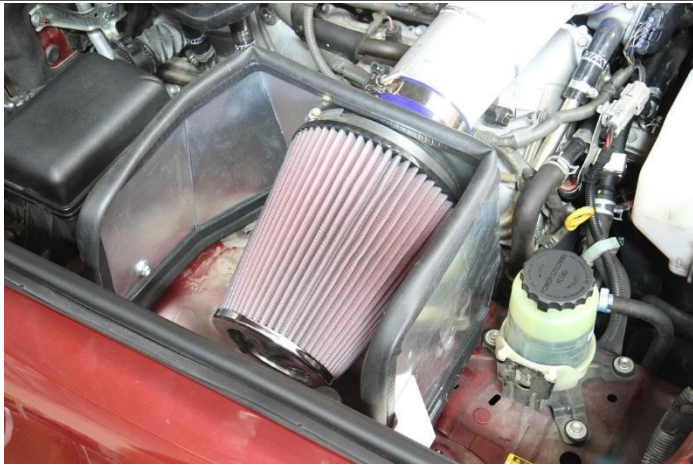
22. Insert the provided HPS air filter onto the velocity stack.
