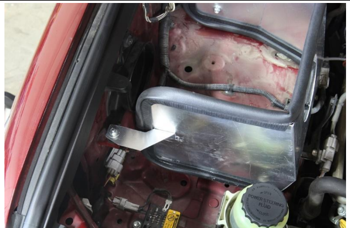
15. Insert the heat-shield into the vehicle. Secure the "L" shaped bracket onto the vibration mount using a m6 nut and washer.
