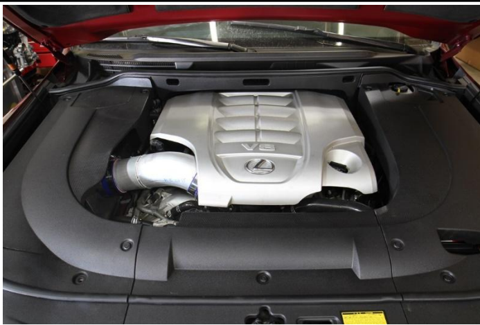
24. Re-install the air box panel cover into the vehicle.
