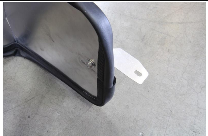
13. Install the "L" shaped bracket onto the left side slot of the heat-shield and secure it using a m6 x 16mm bolt, washer, and nut.
