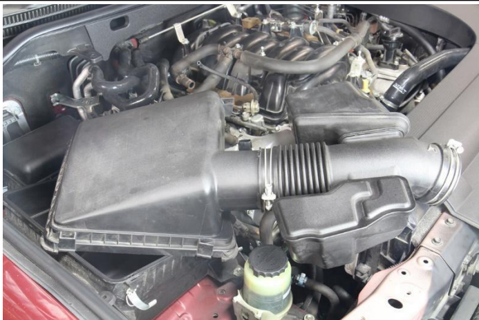
8. Remove the stock intake assembly along with the air box lid from the vehicle.
