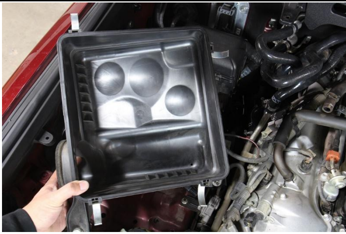
10. Disconnect the air box from the side air scoop and remove the lower air box assembly from the vehicle.
