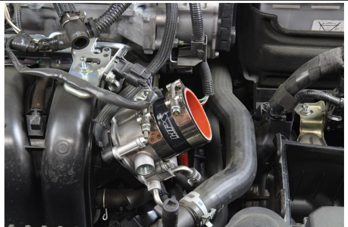
9. Insert the provided silicone coupler along with the t-bolt clamps onto the throttle body.
