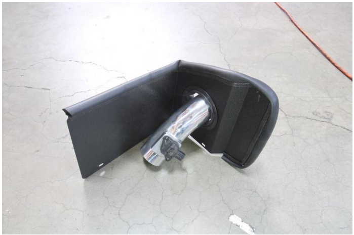
14. Insert the HPS intake pipe into the heat-shield. * This will make it easier to install instead of installing the pipe when the heat-shield is mounted first*
