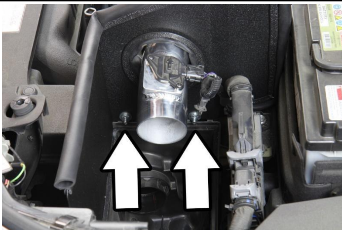
20. Install the M6 flat washers onto the M6x25mm bolts and thread the M6 nuts onto the bolts.
