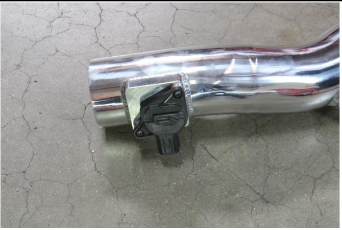
11. Remove the MAF sensor from the stock air box and install the sensor onto the HPS intake pipe. Secure the sensor using the M4 bolts supplied in the hardware kit.
