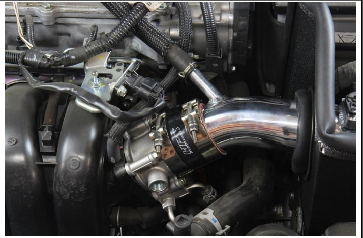
17. Adjust the pipe to the proper position and tighten the t-bolt clamp, then re-install the stock breather hose onto the intake barb.
