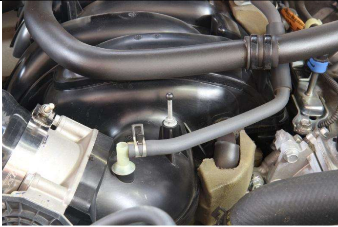
18. Remove the mounting stud from the intake manifold.
