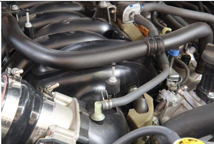
20. Re-install the mounting stud onto the male-to-female rubber vibration mount.
