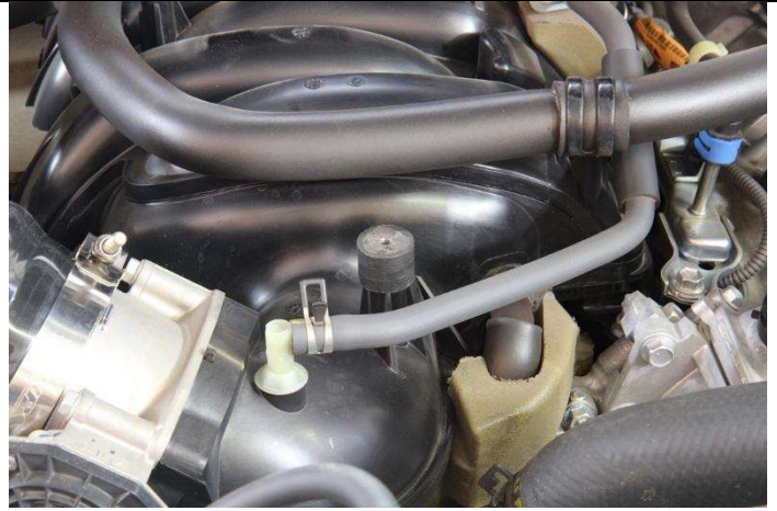
19. Install the male-to-female rubber vibration mount onto the hole that the mounting stud came from.
