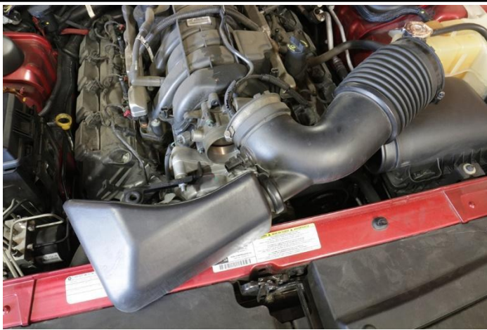
6. Remove the stock intake tube from the vehicle.
