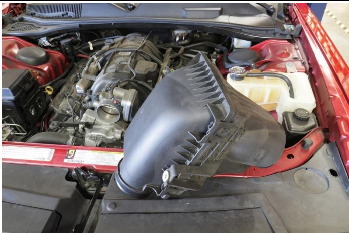
8. Lift and remove the air box assembly from the vehicle.
