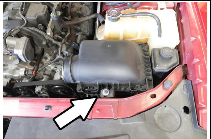
7. Remove the 10mm bolt securing the air box assembly.
