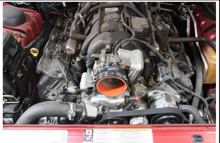
9. Install the coupler along with the provided t-bolt clamps onto the throttle body.
