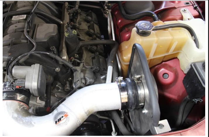
17. Re-install the breather hose onto the intake pipe.
