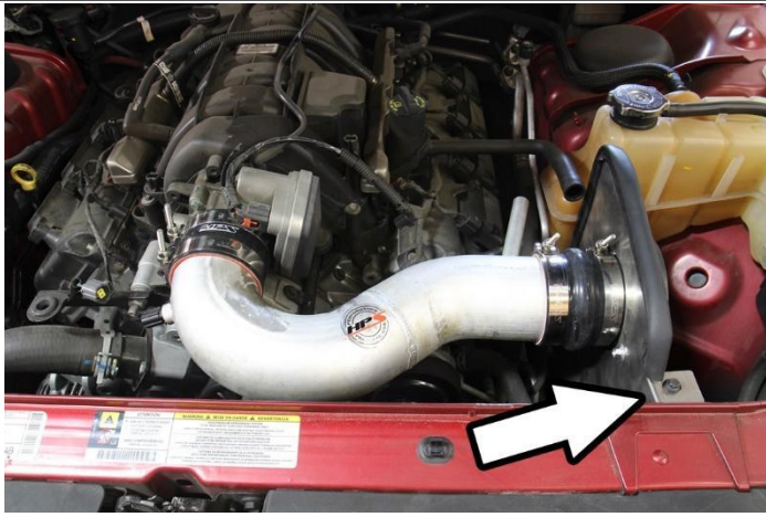
16. Adjust the heat-shield and the intake to the final position and tighten all the clamps, then re-using the stock air box bolt secure the heat-shield to the stock mount.
