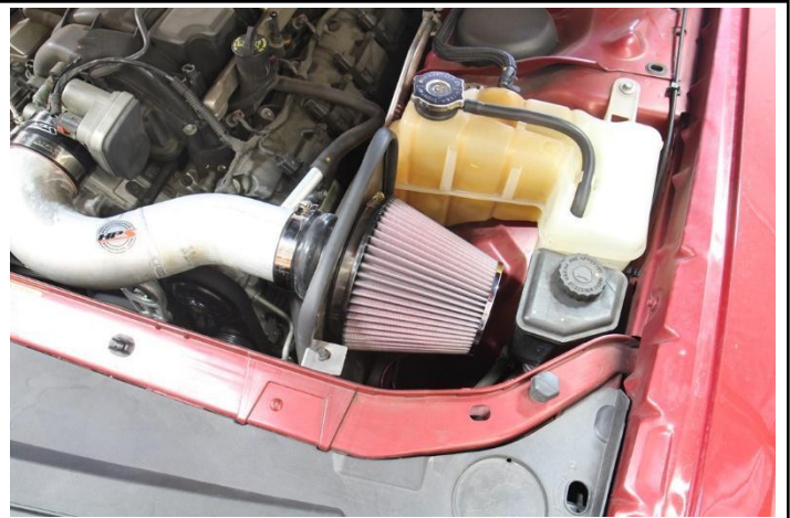
19. Install the provided HPS air filter onto the velocity stack.
