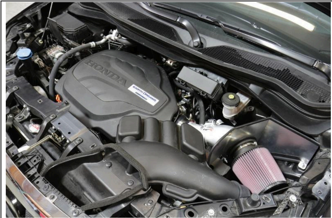
25. Reinstall the air duct and the engine cover back onto the vehicle.
