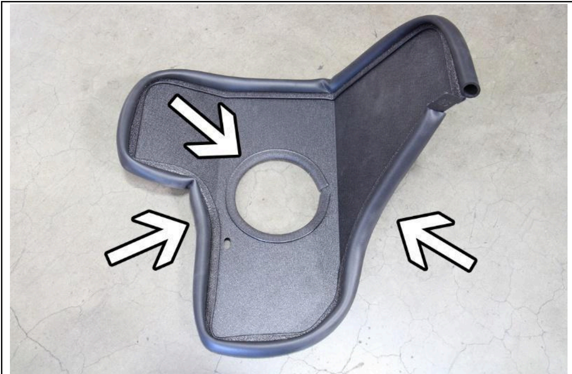
19. Install the bubble edge trim on the outer part of the heat shield and the thin edge trim onto the opening of the heat-shield.
