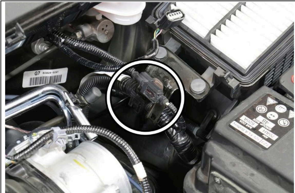
7. Depress each latch and remove the wiring harnesses from the air box bracket.
