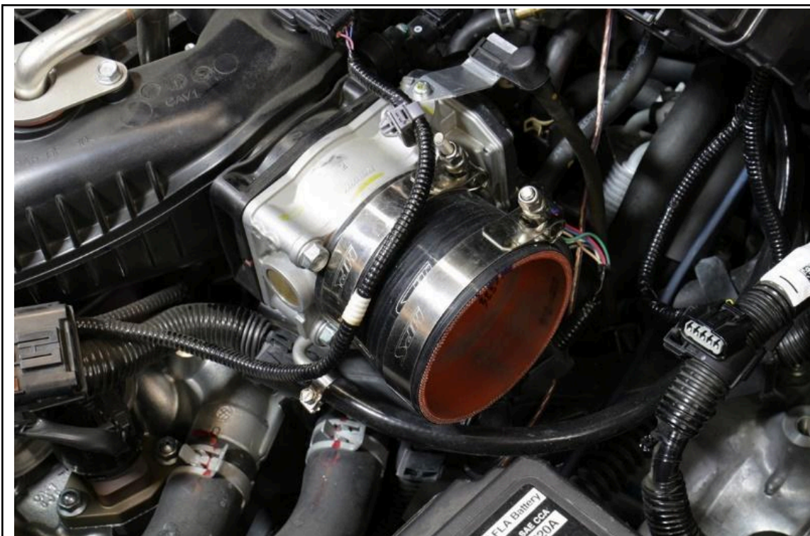
15. Install the reducer coupler onto the throttle body along with the provided T-bolt clamps.
