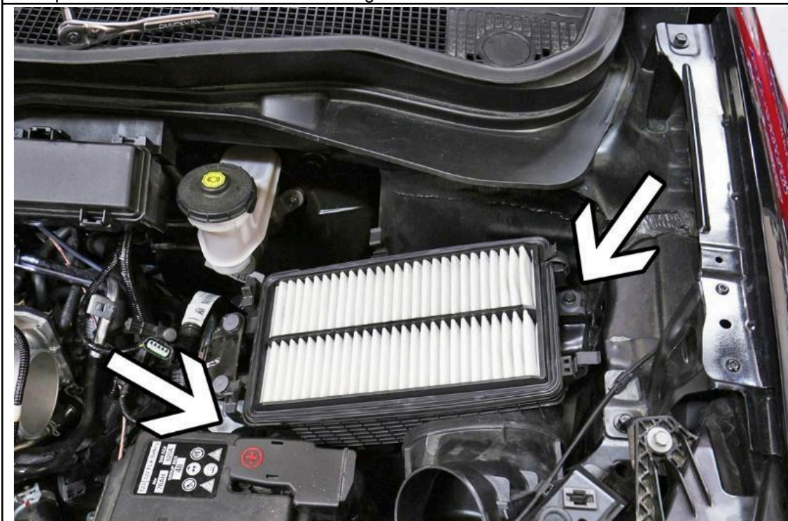
8. Remove the two 10mm bolts securing the lower air box and remove the air box assembly from the vehicle.
