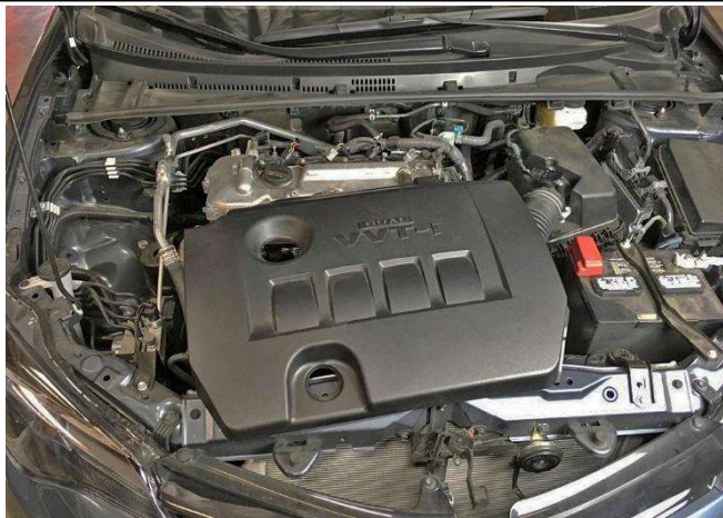
2. Lift and remove the engine cover from the vehicle.
