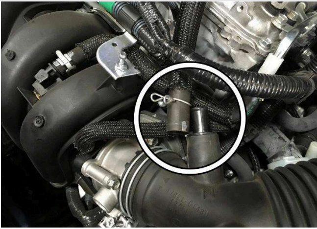
4. Loosen the hose clamp and remove the breather hose from the stock intake tube.
