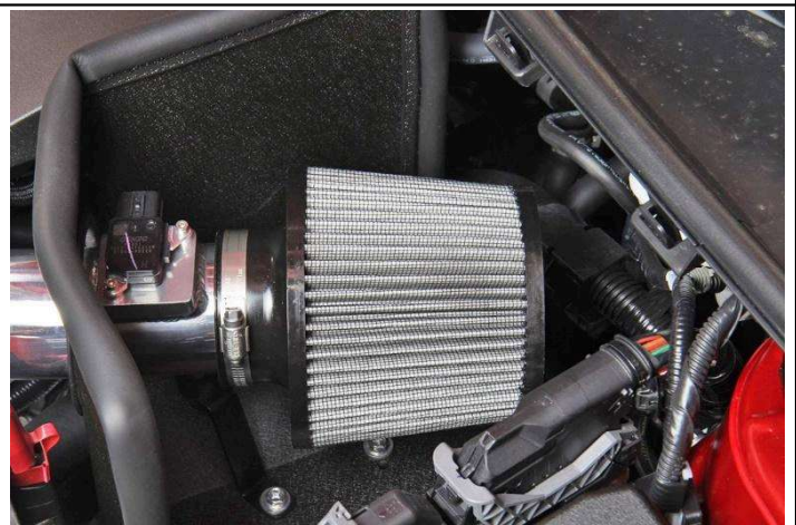
21. Install the HPS air filter onto the HPS intake pipe.
