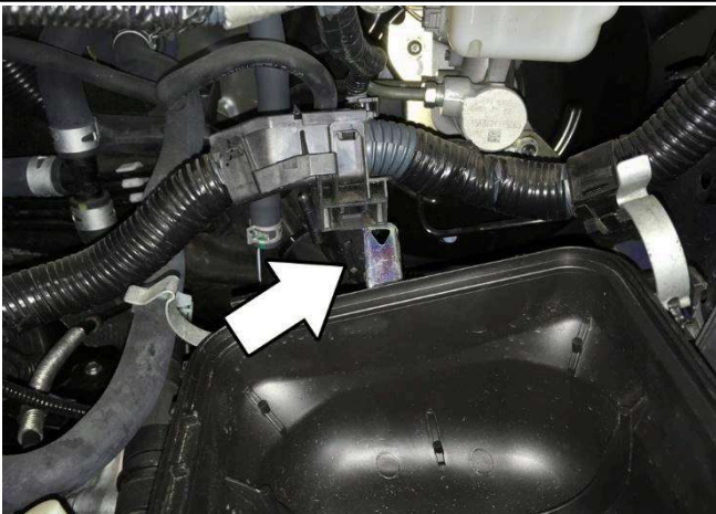
8. Unclip the wiring harness from the rear of the air box.
