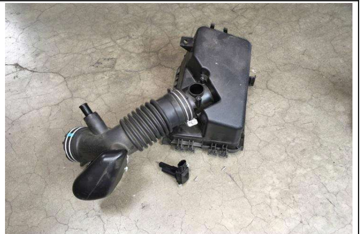
15. Remove the Mass Air Flow sensor from the stock air box.
