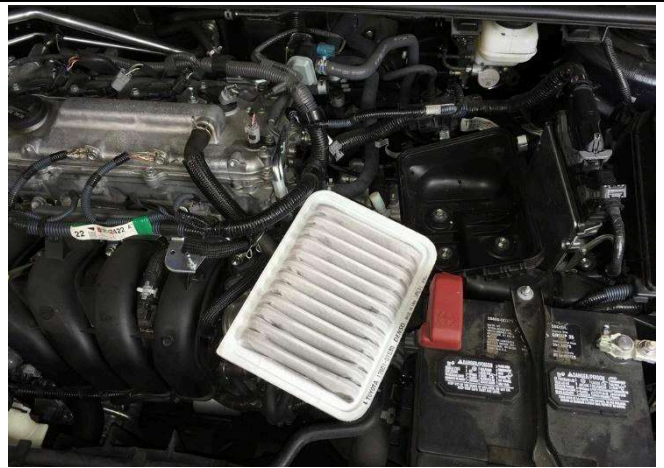
7. Remove the stock air filter from the vehicle.
