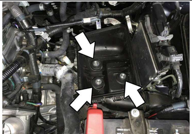
9. Unbolt the three bolts securing the lower air box and remove the air box from the vehicle.
