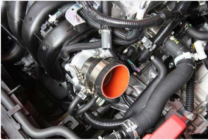
10. Install the reducer coupler along with the T-bolt clamps onto the throttle body.
