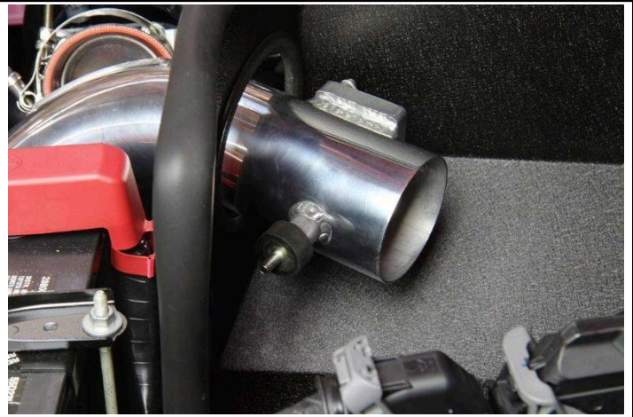
17. Install the rubber vibration mount onto the HPS intake pipe.
