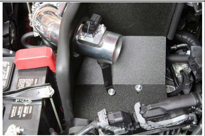
19. Insert the HPS intake pipe into the throttle body coupler and secure the intake bracket onto the heat shield mounting bracket. Tighten the nut on the rubber vibration mount once everything is aligned.
