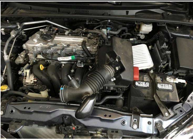
6. Remove the upper air box assembly and the intake assembly from the vehicle.
