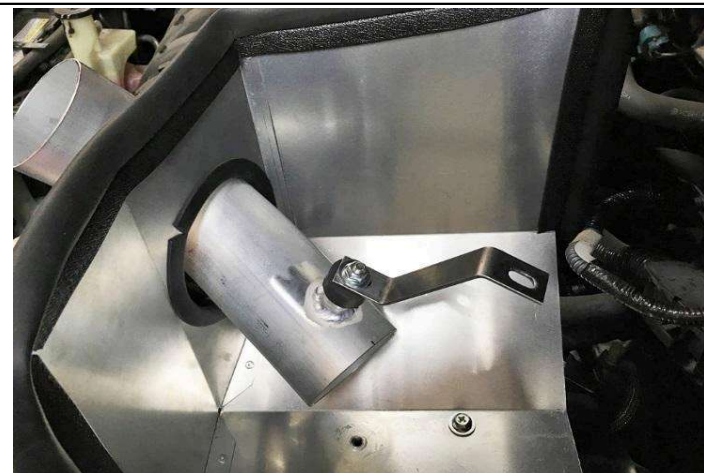
18. Install the intake bracket onto the HPS pipe, but do not tighten the nut all the way.
