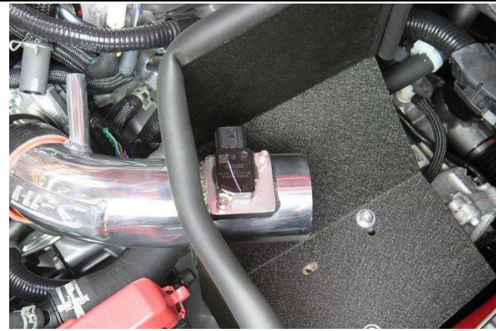
16. Install the MAF sensor onto the HPS intake pipe.
