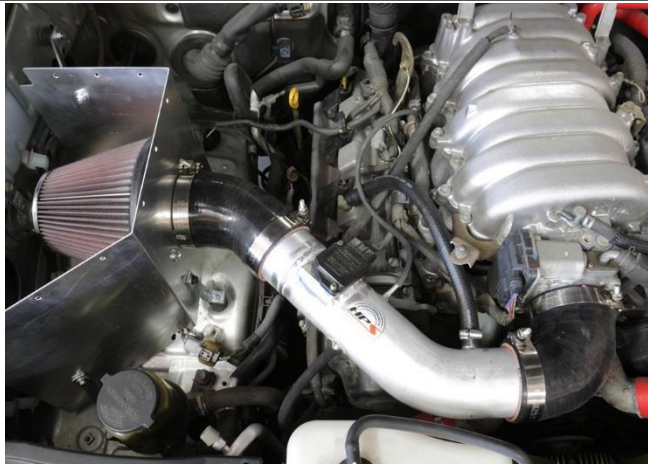
30. Position the intake to the correct position and tighten all the t-bolt clamps to secure the intake pipe.
