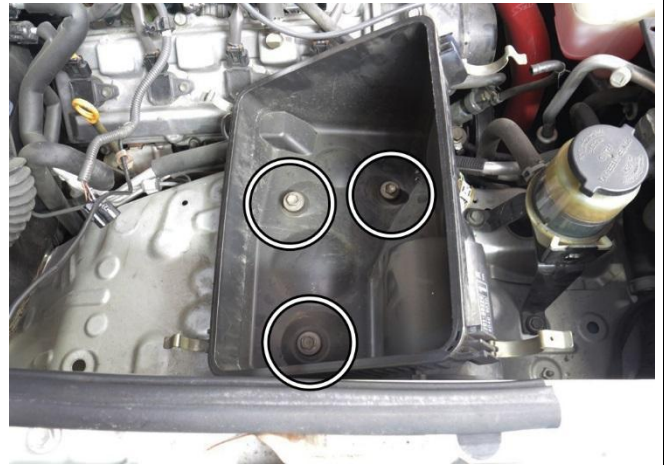
11. Remove the three 12mm bolts holding the lower part of the air box and remove the lower air box from the vehicle.
