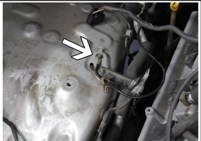
13. Re-mount the ground wire located in the image above.
