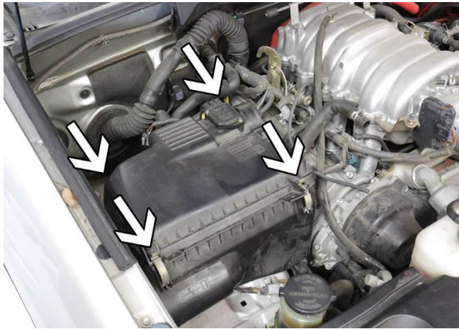
10. Loosen the four retaining clips securing the top portion of the air box and remove it from the vehicle.
