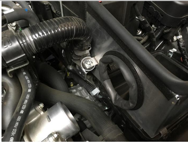
16. Reinstall the nut and tighten all the way. Now you can tighten the nut and bolt for the bracket on the heat shield.
