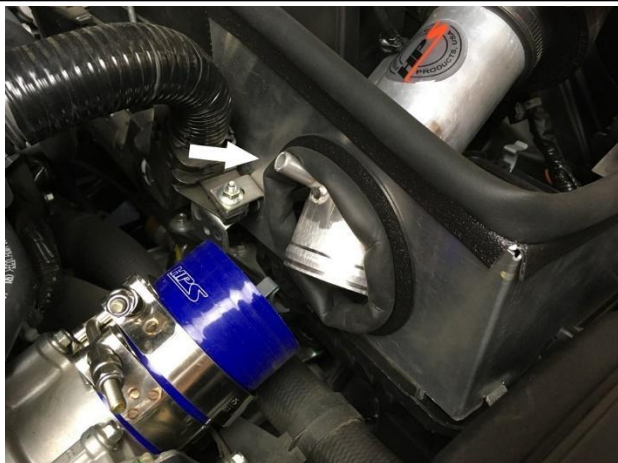
20. Insert the new shortram intake through the heatshield as pictured above.
