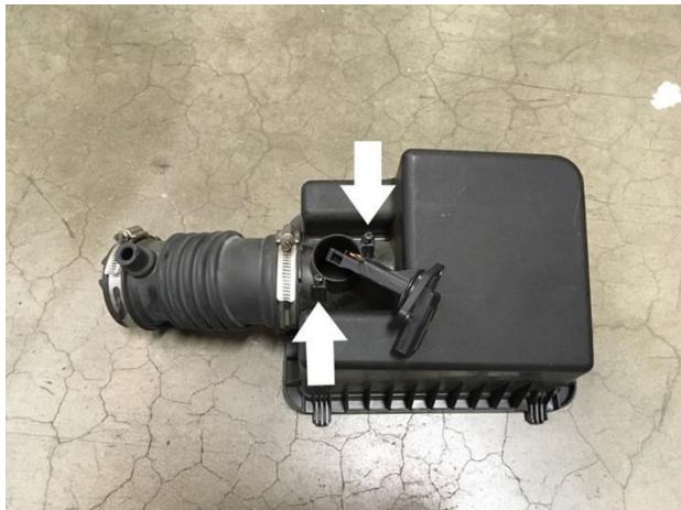
18. Remove the 2 screws holding the MAF sensor onto the factory airbox.
