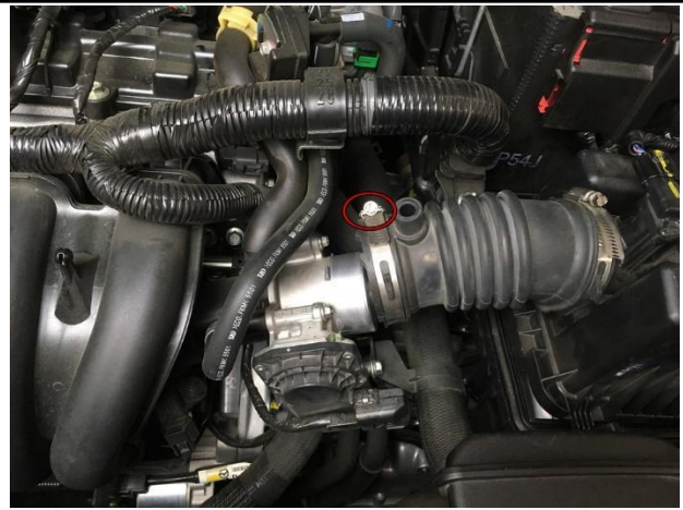
5. Loosen the clamp on the intake tube, then remove it from the throttle body.
