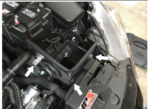
15. Slide the 2 tabs on the heat shield into the OEM location for the upper air box. Rotate the bracket at the rear so that it fits onto the chassis stud.
