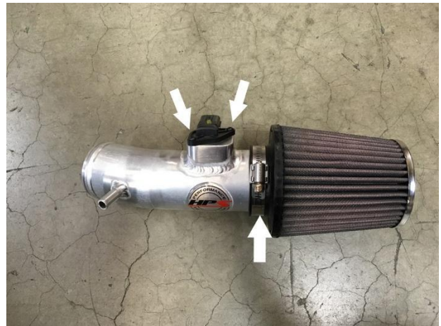
19. Using the provided M4 bolts to mount the MAF sensor to the new shortram intake along with the air filter.
