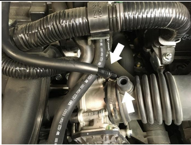
4. Remove the breather barb from the intake tube.
