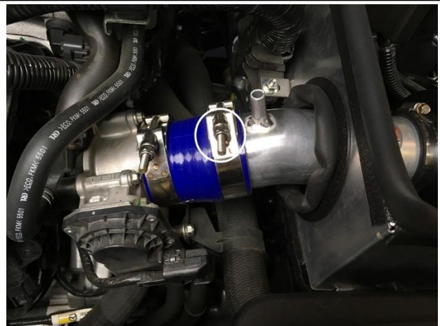
21. Tighten down the clamp circled in the picture above.
