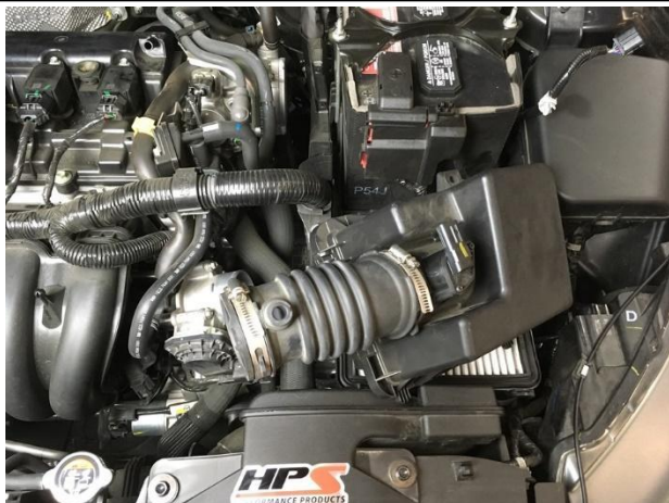
8. Remove the upper airbox from the lower airbox by lifting up on the back side of the airbox and sliding it toward the rear of the car.
