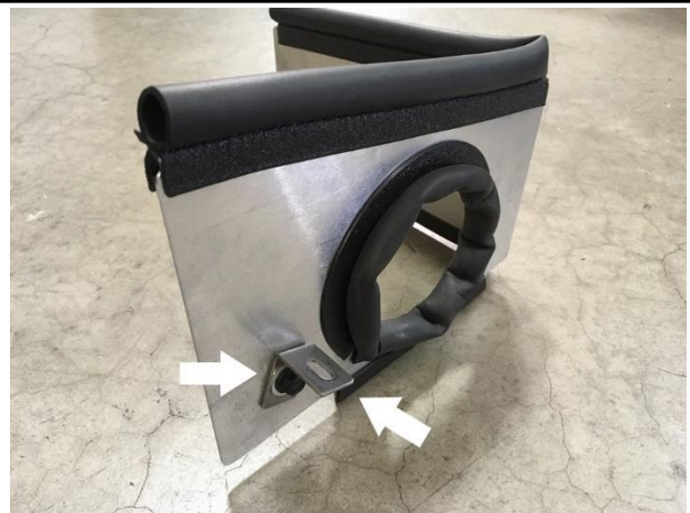
13. Install the provided mounting bracket onto the heatshield with the M6 hardware. Do not fully tighten yet as bracket angle will be found once the heatshield is installed into the car.
