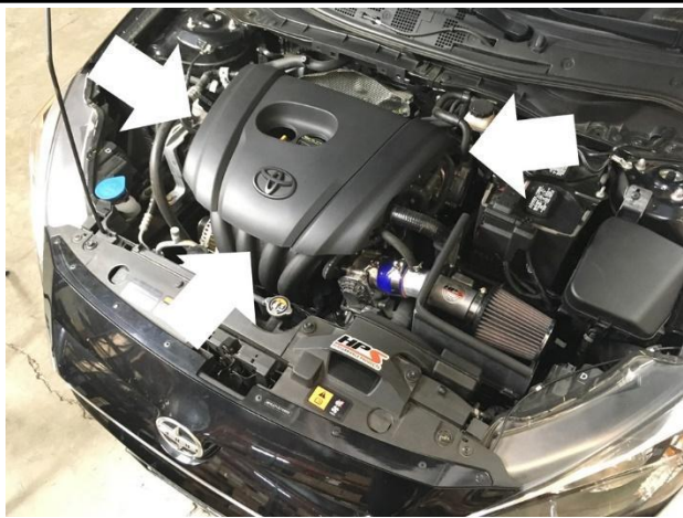
24. Reinstall the engine cover.
