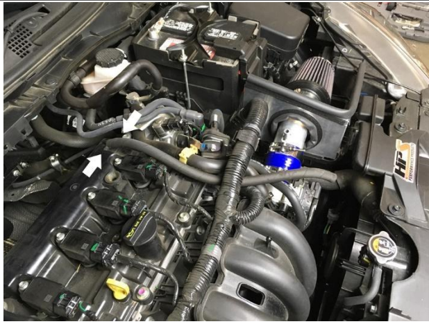
22. Install the provided EPDM hose onto the valve cover breather port.
