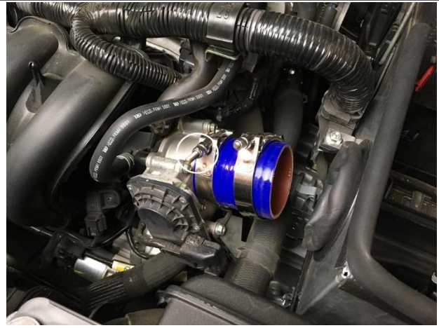
17. Install the coupler onto the throttle body and tighten the clamp circled in the picture.
