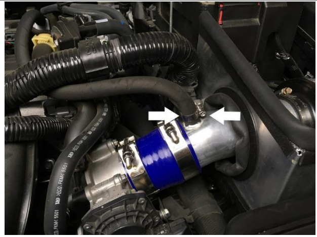
23. Install EPDM hose onto the intake with the provided hose clamp and tighten.
