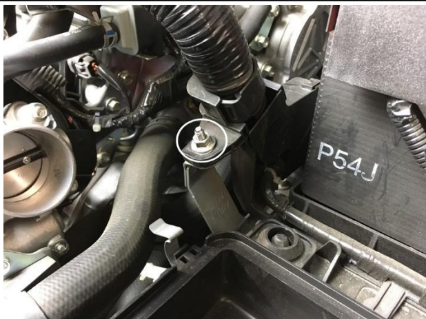
14. Remove the nut circled in the picture above.
