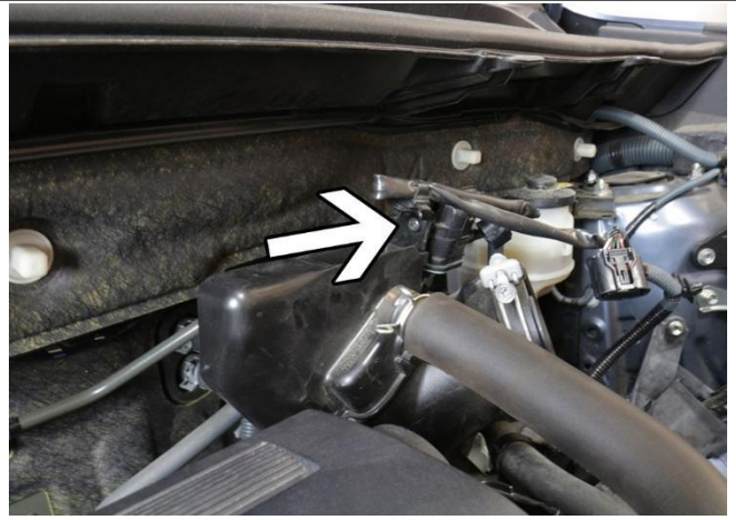
11. Use a Phillips screwdriver to remove the evap. sensor from the intake hose. Save the factory screw for use later in the installation.
