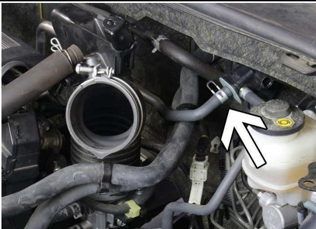
14. Disconnect the evap. sensor hose from the solenoid, then loosen the lower clamp securing the stock intake tube and remove it from the vehicle.
