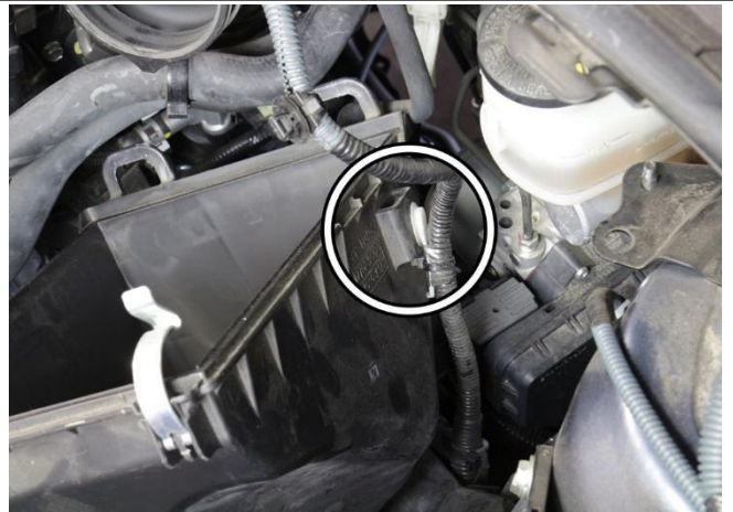
9. Unclip the MAF harness from the lower part of the air box and remove the air box from the vehicle.
