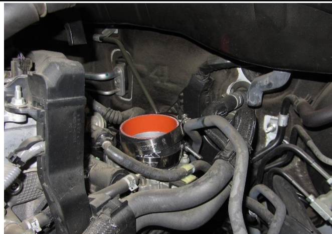
15. Install the HPS coupler onto the throttle body and tighten with the T-bolt clamp included in the hardware kit.
