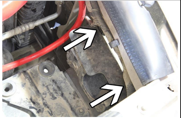
7. Firmly pull and remove the factory air duct from the core support.
