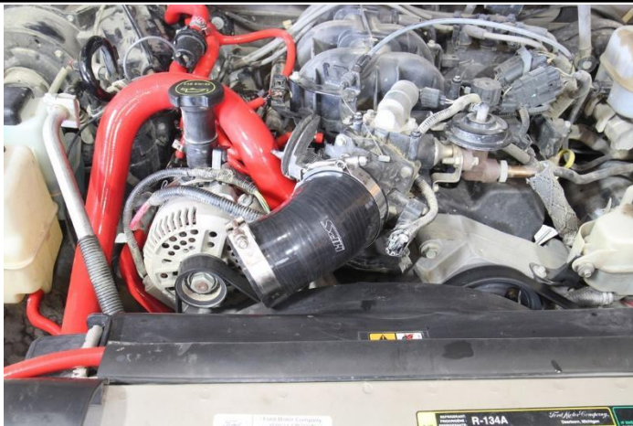
14. Install the 45-degree reducing coupler onto the throttle body along with the provided t-bolt clamps. Do not tighten any of the clamps yet because the coupler will need to be re-adjusted after the pipe is installed.
