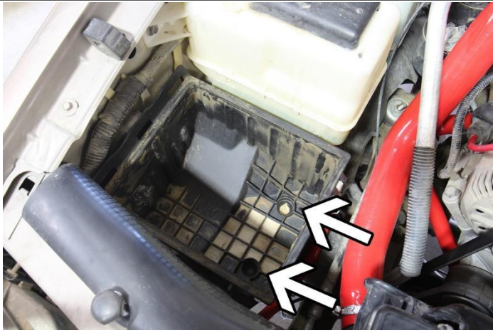
6. Firmly lift and remove the remaining lower part of the air box assembly from the vehicle.
