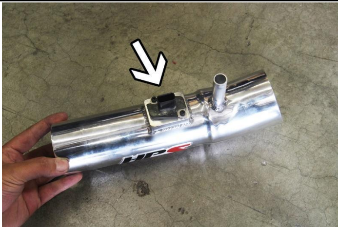
12. Remove the stock Mass air flow sensor and install the sensor into the HPS intake. Secure the MAF sensor using the 4mm Allen bolts provided in the hardware kit.
