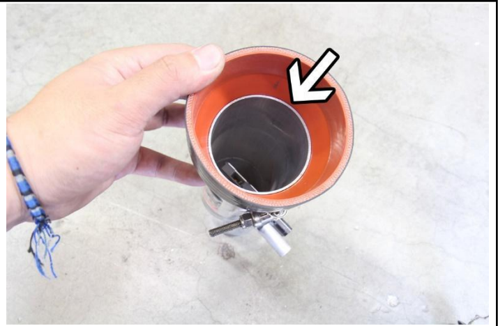
13. Install the reducer coupler onto the smaller side of the intake and secure it using the provided t-bolt clamps. *Make sure when inserting the coupler that the pipe is flush before the reducing part of the coupler.
