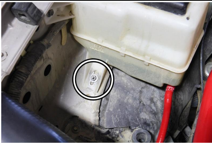
8. Remove the 11mm nut securing the coolant reservoir mounting tab.
