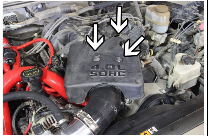
19. Re-install and secure the plastic cover.
