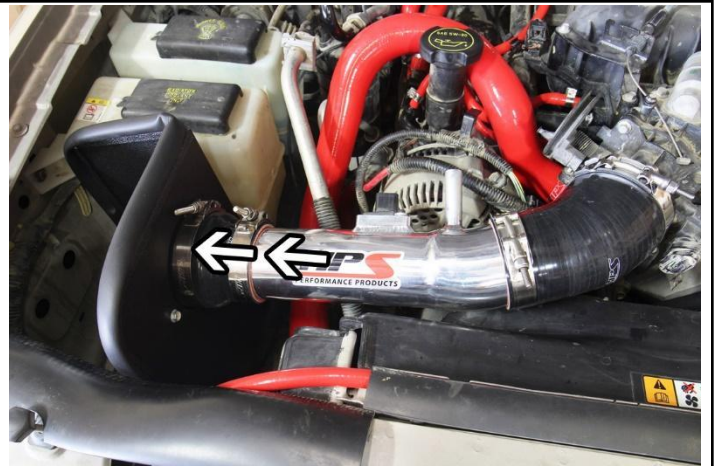
15. Install the intake pipe onto the velocity stack first, then into the throttle body coupler. Adjust the intake pipe and the throttle body coupler to the proper position, then tighten the t-bolt clamps.
