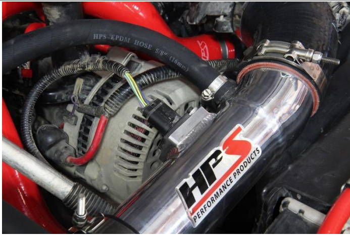
18. Re-connect the MAF sensor connector harness.
