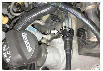
3. Locate the breather hose quick connect fitting located next to the oil fill cap. Slide the locking tab to the right then pull the breather hose forward towards the front of the car.
