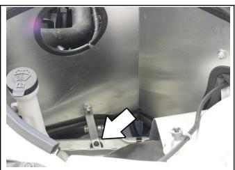
11. Install the heat shield onto the rubber grommet along the frame rail.
