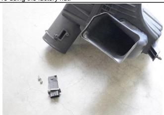
14. Remove the MAF sensor from the factory air box using a 7mm socket.
