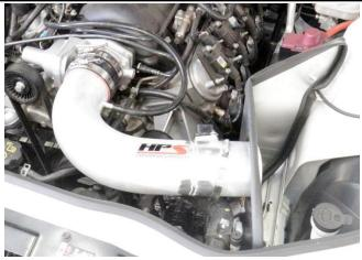
16. Install the intake pipe onto the throttle body. Do not tighten the T-bolt clamp yet as you may need to adjust the position of the pipe.
