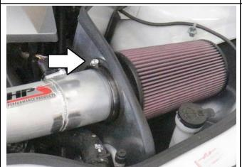
20. Install the new HPS air filter onto the intake pipe. Be sure to place the clamp on the engine side of the heat shield as this will help secure the intake in place.
