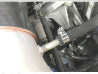
17. Install the provided EPDM hose onto the nipple on the intake pipe and secure it using the FIC clamp provided.
