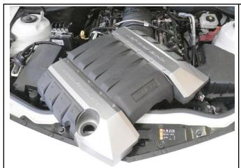
2. Unscrew the oil cap, then remove the engine cover from the vehicle. Re-install the oil cap at this moment to prevent foreign objects from getting into the engine.
