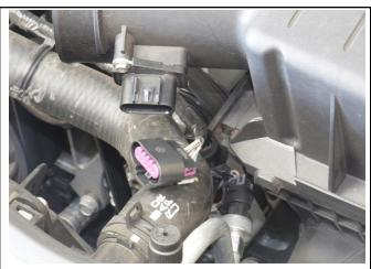
5. Unplug the connector from the MAF sensor.
