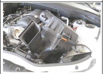
8. Remove the factory air box from the vehicle.
