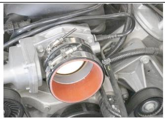
13. Install the silicone coupler onto the throttle body. Secure the coupler to the throttle body using a T-bolt clamp.
