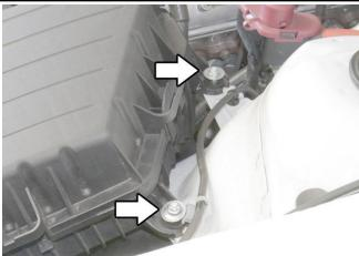
7. Loosen and remove the two nuts holding the air box to the chassis using a 10mm socket.
