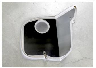
9. Install the thick edge trim along the outside edge of the heat shield and the thin edge trim on the inside hole.
