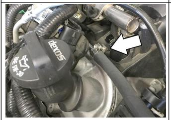
18. Install the opposite end of the EPDM hose onto the factory breather pipe and secure it using the provided FIC clamp.
