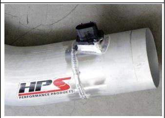
15. Install the MAF sensor onto the HPS intake pipe using the M4 screws provided.
