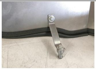
10. Install the grommet mount onto the bracket using a short M6 bolt and washer. Loosely install the bracket onto the heat shield using a medium length M6 bolt, 2 washers and a M6 nut.
