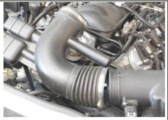
4. Use an 8mm socket to loosen the hose clamps to remove the factory intake tube.
