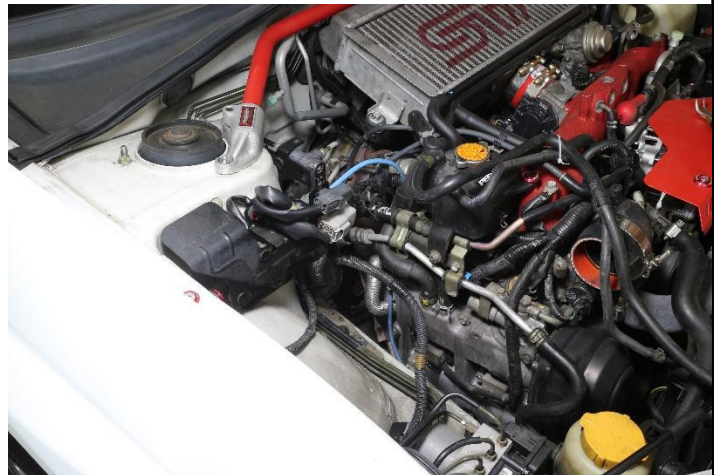
13. Re-insert and clip the electrical connectors back onto the bracket.
