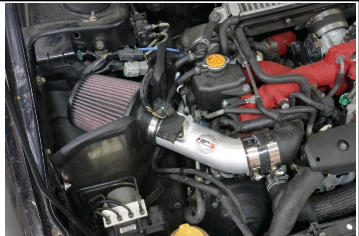
19. Insert the HPS intake pipe into the coupler and align the pipe onto the heat shield. Secure the intake pipe once everything is aligned.
