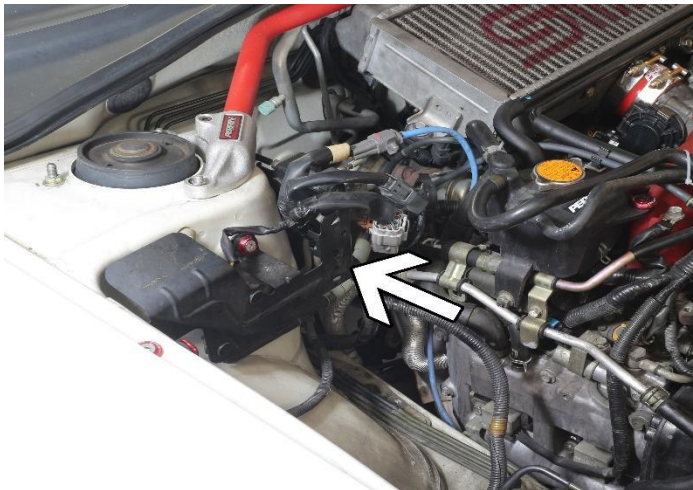
12. Route the harness to the back side of the bracket.
