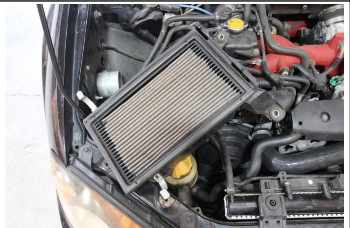
9. Remove the lower air box assembly from the vehicle.
