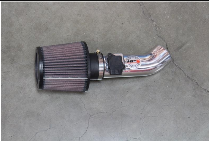
18. Install the provided HPS air filter onto the intake pipe.
