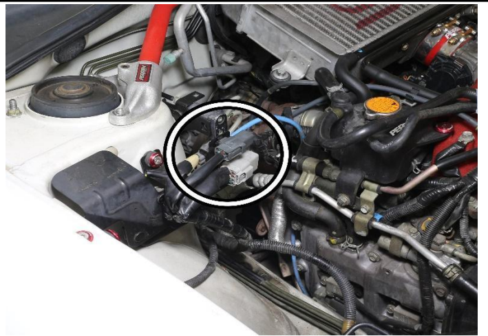
11. Unclip the electrical harness connectors (3 total) from bracket.
