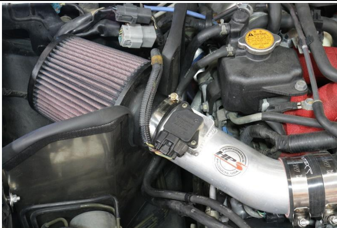
20. Re-connect the MAF sensor connector back onto the MAF sensor.
