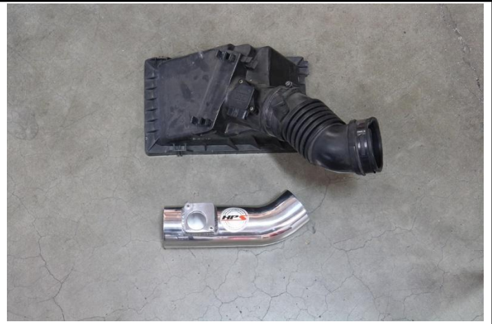
17. Remove the MAF sensor from the stock air box onto the HPS intake. Secure the MAF sensor with the two M4 allen bolts provided in the hardware kit.
