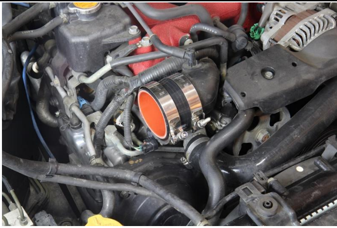
16. Install the straight coupler with the provided T-bolt clamps onto the turbo inlet.
