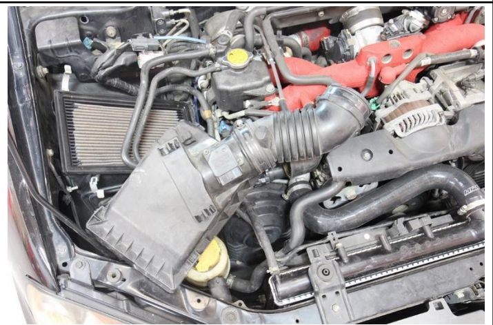
7. Remove the upper intake assembly from the vehicle.
