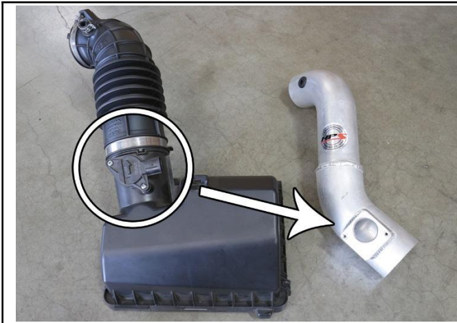
16. Remove the MAF sensor from the factory air box, then install it onto the HPS intake pipe using the M4 screws supplied.
