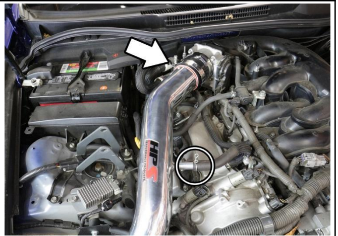
25. Re-install the breather hose onto the HPS intake and tighten the t-bolt clamp securing the intake into the coupler.
