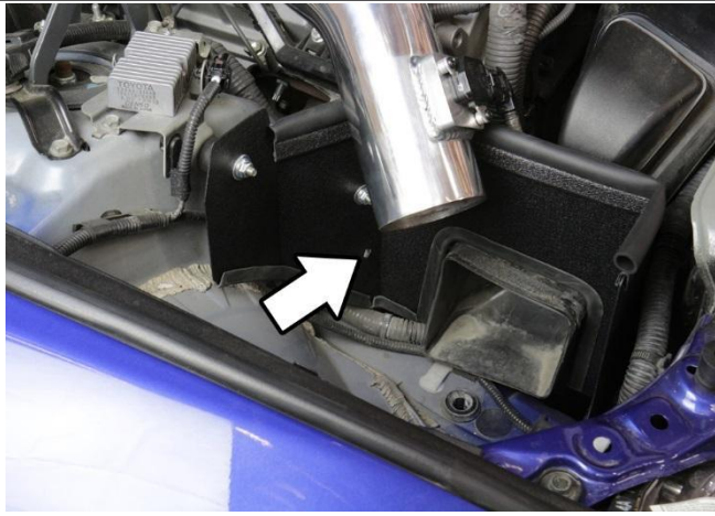
22. Re-insert the MAF sensor harness clip onto the heat shield.
