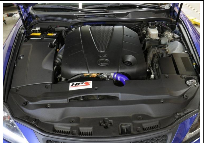
27. Re-install the engine cooling panel as well as the air filter box panel back onto the vehicle.
