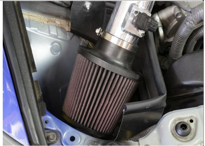
23. Install the HPS air filter onto the HPS intake.
