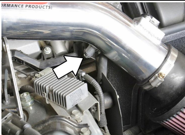
24. Secure the HPS intake pipe onto the bracket using the M6 bolt and washer supplied in the hardware kit.
