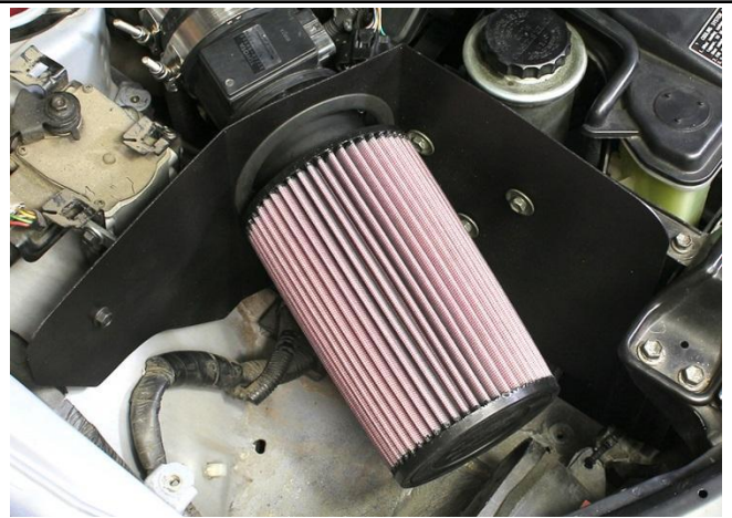
25. Install the air filter and secure the clamp onto the air flow meter.
