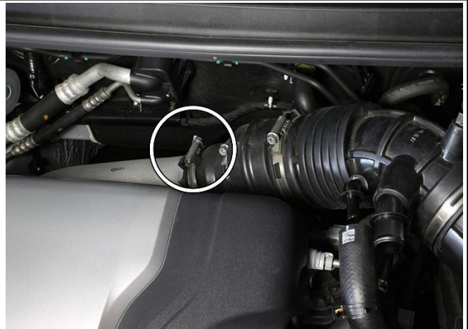
7. Loosen the hose clamp on the turbo inlet.
