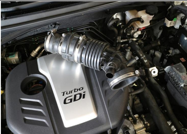
8. Remove the stock intake tube from the vehicle.
