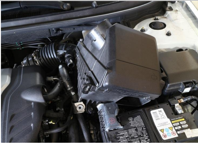
6. Disconnect the intake tube from the air box and remove the air box assembly from the vehicle.
