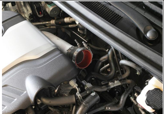
9. Install the reducer coupler with the provided t-bolt clamps onto the turbo inlet.
