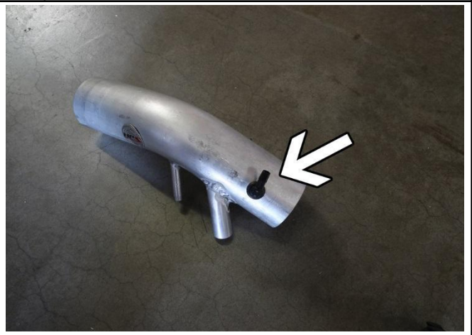
11. Install the rubber grommet along with the 90 degree barb included in the accessory kit.
