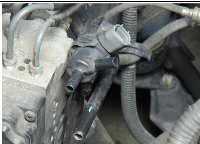
15. Install the EVAP solenoid onto the ABS module and secure it using the nut removed from the previous step.
