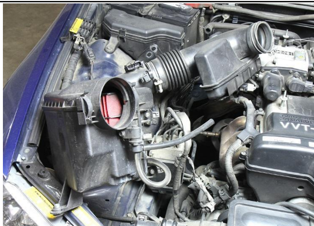
11. Remove the stock air intake assembly from the engine bay.
