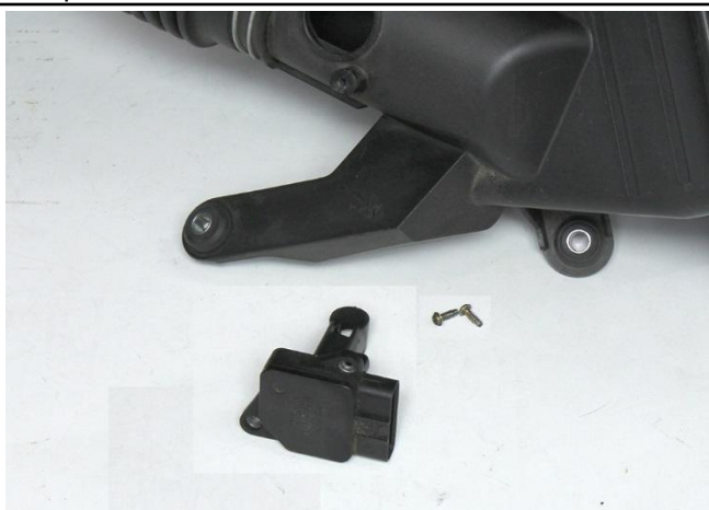
24. Remove the MAF sensor from the factory air box.
