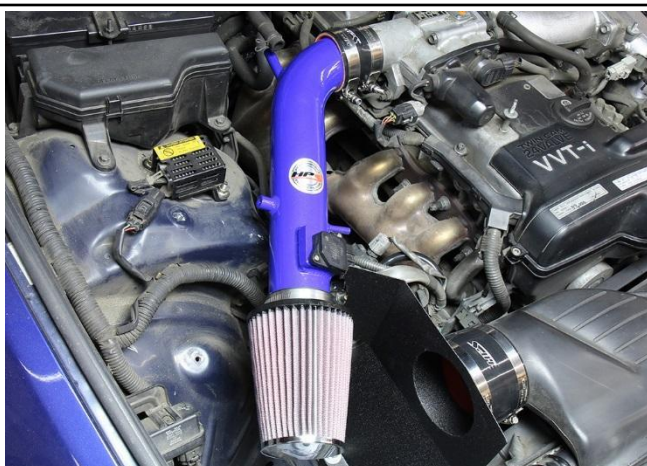
26. Install the HPS air filter onto the air intake pipe then connect the intake pipe to the throttle body. Do not tighten the clamp to the pipe yet.
