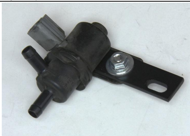
13. Mount the bracket onto the EVAP solenoid.
