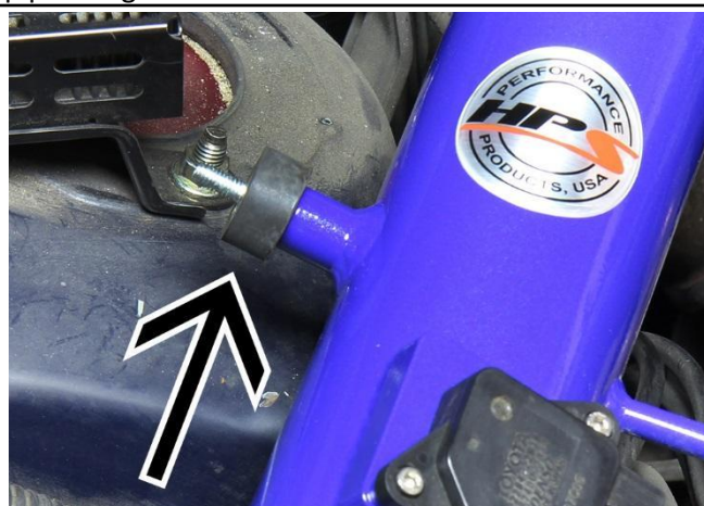
27. Install the short rubber mount onto the threaded bung on the intake pipe.
