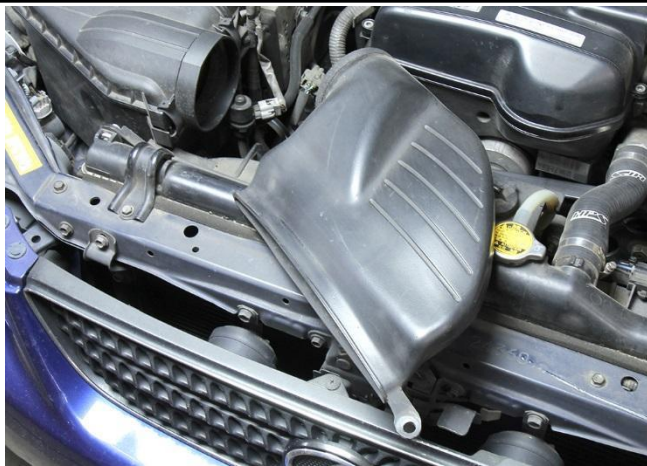
4. Use a 10mm socket to remove the stock air duct.
