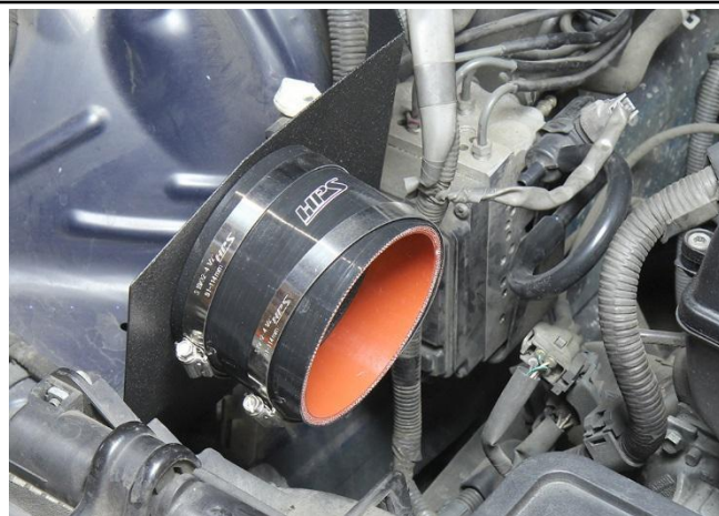
21. Slide on the 4" coupler and hose clamps onto the heat shield.
