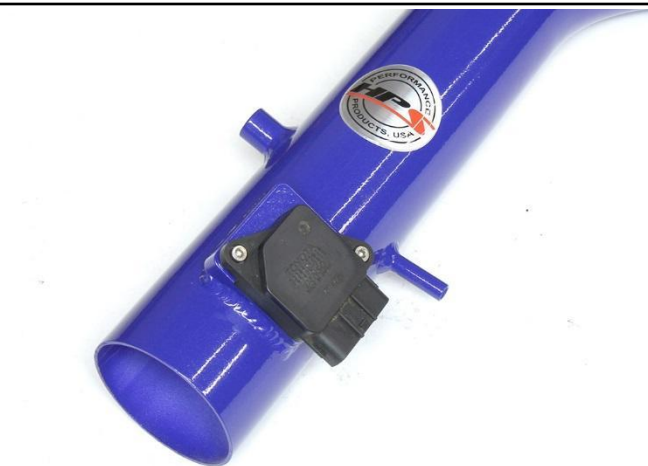
25. Install the MAF sensor onto the HPS air intake pipe using the M4 Bolts included in the hardware kit.
