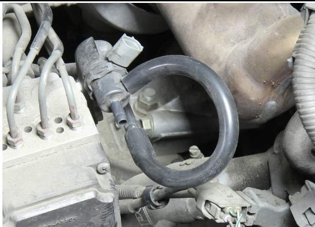
16. Install the 9" long vacuum hose included in the hardware kit onto the EVAP tube and the EVAP solenoid as shown.
