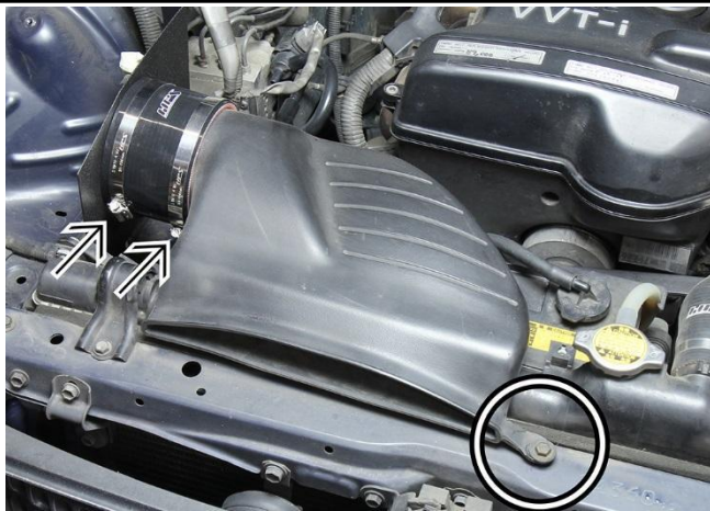
22. Slip on the factory air duct onto the 4" coupler, then secure it using the factory bolt. Tighten the hose clamps.
