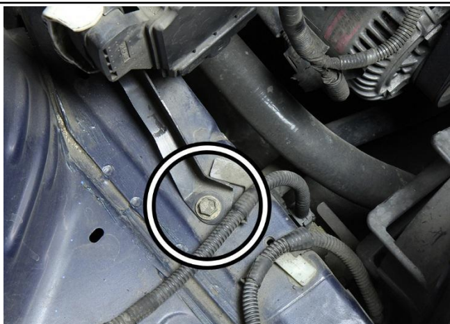
18. Remove the bolt securing the ABS module to the chassis using a 12mm socket.
