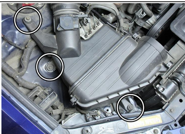
6. Remove the 3 bolts that secure the air box to the chassis.
