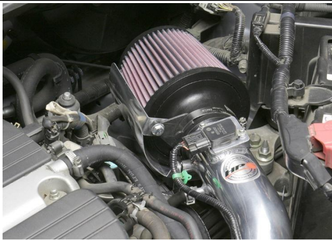
18. Install the air filter and heat shield onto the intake pipe.
