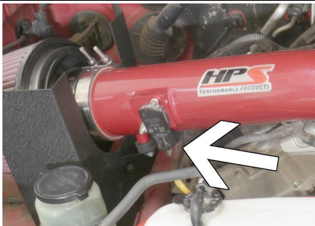
22. Re-connect the MAF sensor harness and install the engine cover onto the vehicle.
