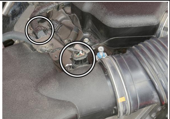
3. Disconnect the Mass Air Flow sensor and the wiring harness from the air box.
