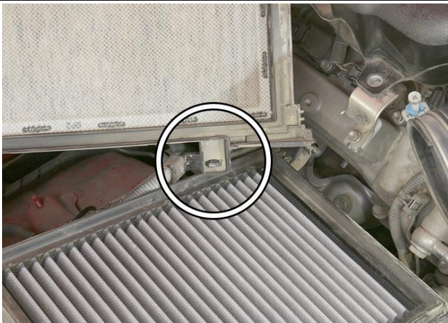
8. Unclip the wiring harness from the air box then remove the upper air box from the vehicle.
