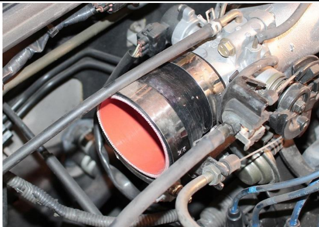
9. Install the reducer coupler and T-bolt clamps onto the throttle body.
