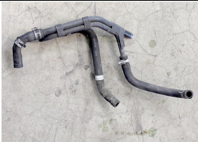
7B. This is the breather/coolant tube that will come off of the engine.
