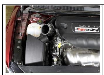
2. Loosen the hose clamp on the intake hose, then detach it from the air box.
