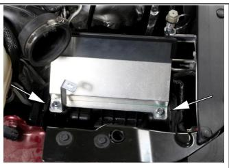
5. Install the HPS heat shield and intake bracket onto the air box sub assembly using an 8mm bolt, 2 washers, and a 8mm nut for each hole.
